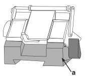
The Finesse 325 microtome has the Coarse advance knob fitted towards the back of the left hand side panel of the instrument. The Coarse Advance knob turns clockwise for specimen advancement.
