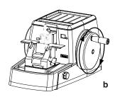
Return the handle to the 12 o'clock position and apply the brake when sectioning is finished. The LCD counter displays the number of cutting cycles performed within the range 1-99. Press the small button adjacent to the display to reset the counter.
