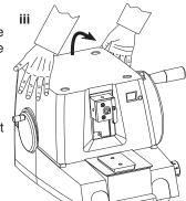
Unscrew and remove the Horizontal and Vertical tilt adjuster knobs.
