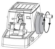
The specimen is retracted from the knife edge during the return stroke to prevent the specimen brushing against the back of the knife blade.
