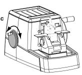
When maximum travel is available, use the Knife Holder Clamp Lever (d) to loosen the knife holder on its carriage. Move the knife as close as possible to the specimen without actually being in a position to make a cut during the first cutting stroke. Push the Knife Holder Clamp Lever away from you to lock the knife in this position.
