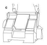
Place the Flip-Up Knife Guard over the blade. Hold the Knife Guard (c) by its two flanges and slide it sideways until the blade engages between these flanges. Use the
