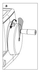
If necessary release the brake and rotate the handwheel until the handle is just at the 1 o'clock position, then re-apply the brake (a).
