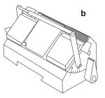
Slide the blade a sufficient distance from its dispenser to enable one end to be inserted in the Knife Holder, then withdraw the dispenser leaving the blade in position (b).
