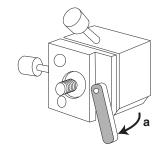
Fit the Specimen Clamp on the threaded bolt at the end of the Orientation Head, then screw it clockwise to tighten it in position (b).
