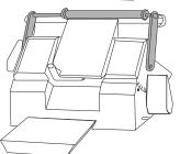
The Knife Guards of the Universal Knife Holder comprise two platforms - one either side of the cutting aperture. They require no adjustment or setting up.
