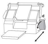
During normal operation the specimen advances by the distance set by the Section Thickness Control (b) as each successive section is cut. The maximum travel available is 16mm. During the course of specimen travel the indicator shows red with green when travel is available in both directions.
