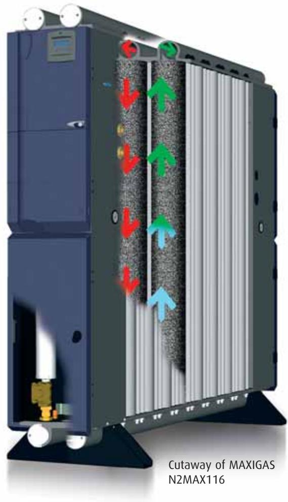
After a pre-set time when the on-line bed is almost saturated with adsorbed gases, the system automatically switches the bed to regenerative mode, venting the contaminants from the CMS. The second CMS bed then comes on-line and takes over the separation process. The pair of CMS beds switch between separation and regeneration modes to ensure continuous and uninterrupted nitrogen production.
