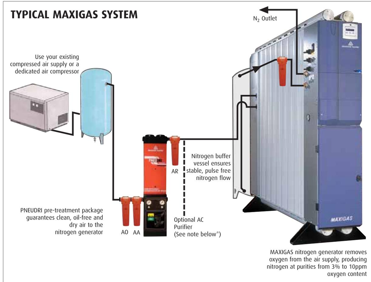
\*Note: In high ambient temperature applications, it may be necessary to install an additional activated carbon stage to protect the nitrogen generator from oil vapour carryover. Please consult domnick hunter for advice.
