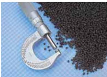
Carbon molecular sieve differs from ordinary activated carbons in that it has a much narrower range of pore openings. This allows small molecules such as oxygen to penetrate the pores and be separated from nitrogen molecules which are too large to enter the CMS. The larger molecules of nitrogen by-pass the CMS and emerge as the product gas.
