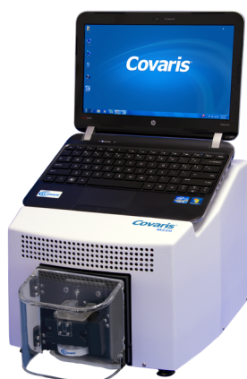
Figure 2.2 Secure the computer on top of the M220 as shown.
