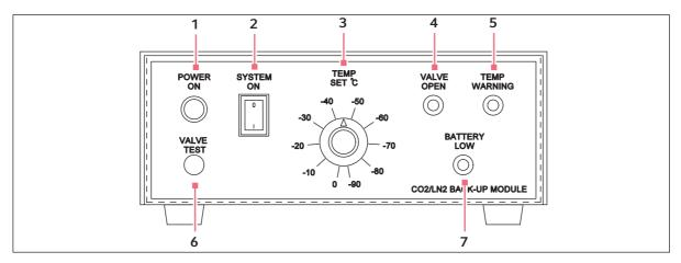
Fig. 3-1: Front view of the CO<sub>2</sub> Back-up System
