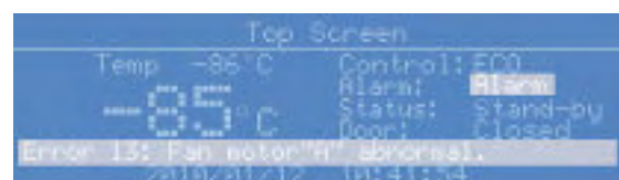
Out-of-compliance events are announced by visual and audible warnings. Error codes quickly identify problem sources and permit fast diagnosis and remediation.
