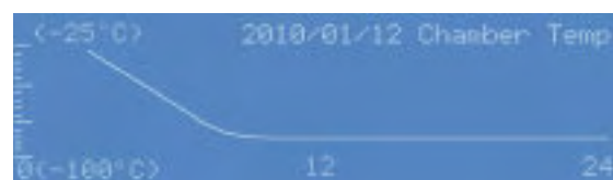
Internal temperature log files are displayed in graphical form over time.
