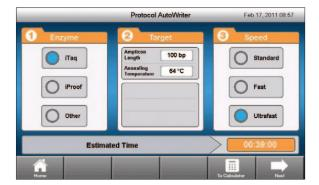
Quick and easy protocol programming. The protocol autowriter in the cycler's onboard software can automatically suggest a fast temperature protocol based on input parameters. Suggested protocol is based on standard PCR guidelines, with hot-start, initial denaturation, annealing, and extension steps. Further reductions of run times are achieved by minimizing the number of steps and cycles, incubation times, and temperature differentials.
