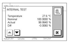
You can use the internal weight to check the correct adjustment of your balance by pressing this function key.
