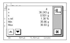
The statistical window contains the result of the series of weighings. (The information that you selected for printing the result is displayed, see Section 7.3.4). Please note the information in Section 7.4.3 regarding units, readability and the precision of the displayed values.
