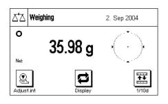
**Weighing:** Place the items to be weighed on the weighing pan, and close the glass draft shield (if present). As soon as the stability detector icon (the small circle to the left of the weight display) goes out, the display is stable and you can read off the weighing result. The stability detector icon is still visible in this diagram, and therefore the weighing result is not stable.
