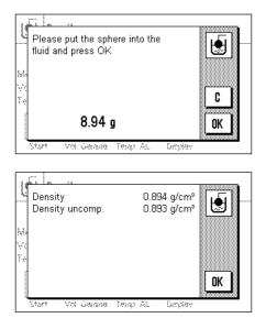
When the sample has been tared, you will be prompted to submerge the gamma sphere in the sample substance.
