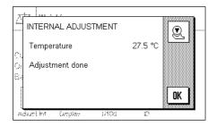
Pressing this function key triggers an adjustment of the balance using the built-in adjustment weight. You can do this at any time; you can also specify in the system settings that the balance requests adjustment as soon as a specified change in ambient temperature has taken place (*Callno* setting, Section 5.3.1).
