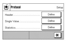
Additional settings for density determination, described below, are available in the three submenus in which you can specify the options for the printout header, for printing the individual values, and for the statistical printout.
