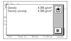
The balance now determines the density of the solid body, and then displays the result (the compensated and/or uncompensated value, depending on the settings that you have made for output of the result, see Section 9.3.5).
