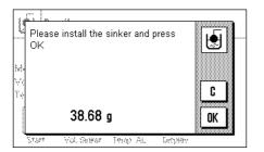
Press the "**Start**" function key to start the density determination. You are prompted to attach the sinker (weighing in air for taring).
