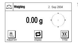
The display shown here appears the first time the balance is switched on.
