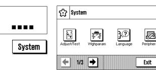
**Change system settings:** If you want to change system settings that apply to the entire weighing system, i.e. to all the applications, then press the «....» key and then the **"System**" button. The system settings are described in detail in Section 5.
