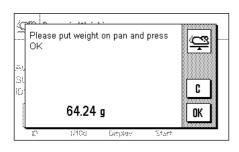
Press the **"Start**" function key. If the "AutoTare" function is activated, the display is automatically set to zero. You will then be prompted to place the weighing object on the balance. When you have done this, press the **"OK**" button to start the measurement. As soon as the value becomes stable, the weight is accepted.
