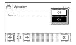
Automatic zero setting ("AutoZero") continuously corrects possible variations in the zero point that might be caused through small amounts of contamination on the weighing pan.
