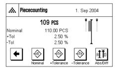
When you have entered the target value and tolerances, the tolerance marks for the "SmartTrac" graphical weighing aid appear in the display. The tolerance marks make weighing to the target value easier. You can weigh your samples roughly until the lower tolerance value is reached, and then dispense finely to the target value.
