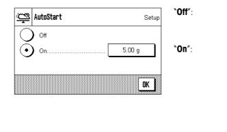
No automatic start. Each measurement cycle must be started **manually** and the "**Start**" function key must be active (Section 13.3.2).
