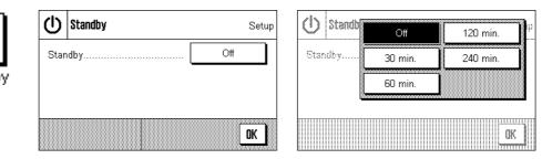
You can switch the energy saving function off ("Off"), or you can specify a period of 30, 60, 120 or 240 minutes after which the balance is to switch itself into standby mode. The standby mode is the same state into which the balance enters when switched off with the **«On/Off»** key. The **«On/Off»** key must be pressed to turn the balance on again.
