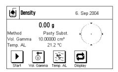
Please put sample on pan and press OK VC Te 10.44 g Start Vol Ganaa Tenap AL LacpBay In the application-specific settings, select "Pasty Subst." as the method (Section 9.3.2).
