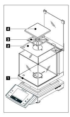
XP precision balances with readability of 1 mg, S platform with draft shield
