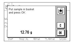
The result of the weighing is stored, after which you are prompted to immerse the solid body in the auxiliary liquid.
