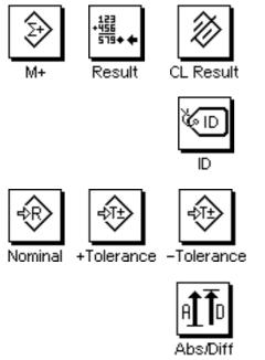
At least the three function keys "M+", "Result" and "CL Result" must be active for Formulation (Section 8.3.2).
