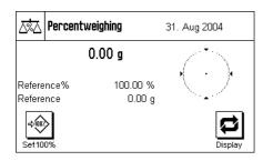
After you have selected the application, the display shown at left appears. Some of the special function keys and the special information fields for percent weighing are activated at the factory. How you can adapt these, and other, settings to your needs is described in the Sections that follow.
