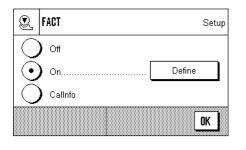
You can make the settings for fully automatic adjustment using the internal adjustment weight in this menu (FACT). FACT (Fully Automatic Calibration Technology) calibrates the balance under full automatic control on the basis of a pre-selected temperature criterion.
