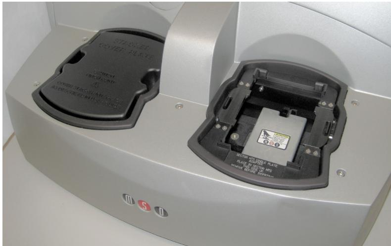
6. Load the SECTOR Imager demonstration plate into the single plate adaptor (Figure 5:7). (Sensors in the instrument will automatically identify the plate orientation and adjust the data acquisition and analysis accordingly.)
