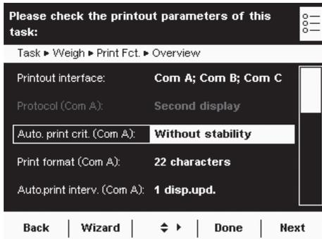
▷ At a preset interval, automatic printouts should be sent to the connected peripheral device as a second display.
