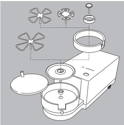
**Filter Balances (models MSU6.6S-F/2.7S-F): Placing Components on the Weigh Cell**
