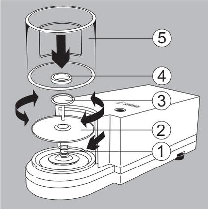
**Models MSU6.6S/3.6P/2.7S: Placing Components on the Weigh Cell**
