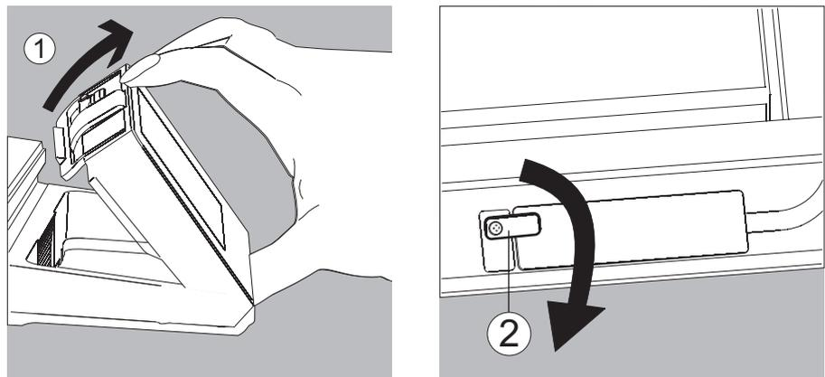
1. Tilt the control unit until it is nearly vertical.
