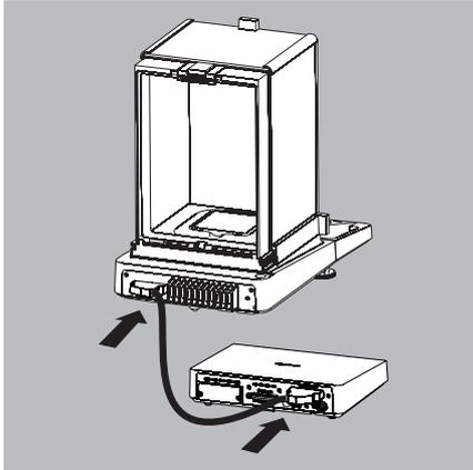
**Models with an External Electronics Module: Connecting the Weigh Cell to the Electronics Module**
