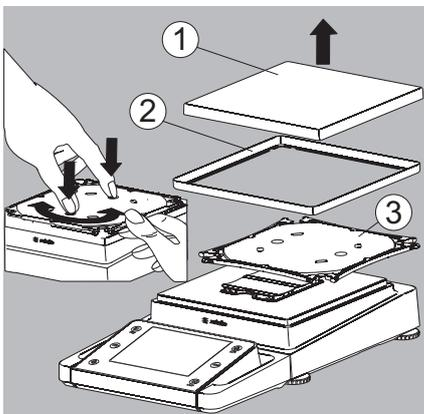
**Removing the Display and Control Unit from Precision Balances without a Draft Shield with a Weighing Range of up to 15 kg**
