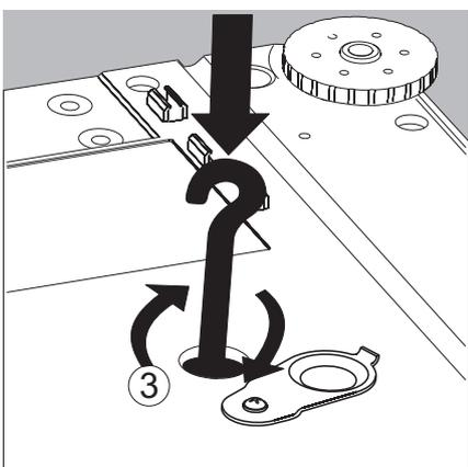
3. Carefully screw on the hook for below-balance weighing.
