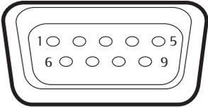
**Pin assignment 9-pin socket, RS-232:**
