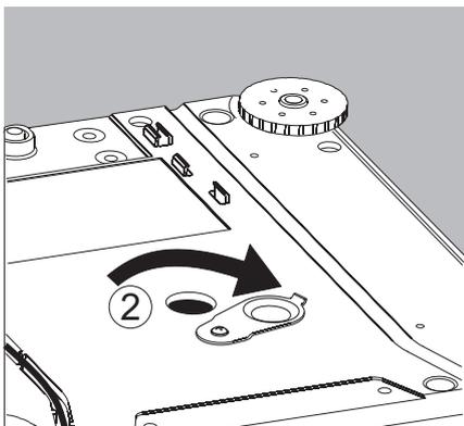
2. Push the cover of the below-balance weighing port to one side.
