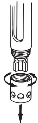
**Fig.12 Changing the Stator - Tubular Mixing Assemblies**
