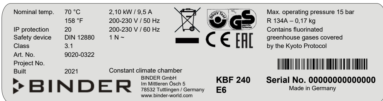
Figure 3: Type plate (example KBF 240 regular chamber 9020-0322)
