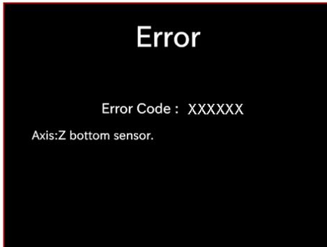
Error code reported is shown in place of “XXXXXX” in the above screen and the corresponding error message is displayed under the code. Refer to Section XII, “List of Common Error Codes” for a list of common error codes and countermeasures to be taken.
