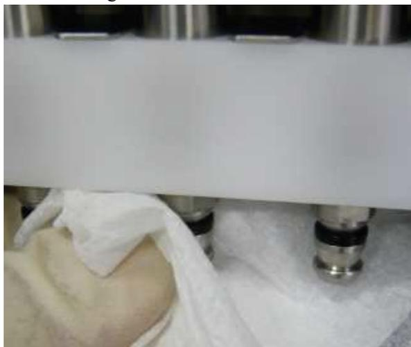
2. Wear gloves and put a small amount of silicon grease on your fingertip. Then spread silicon grease by rubbing it on the O-rings.
