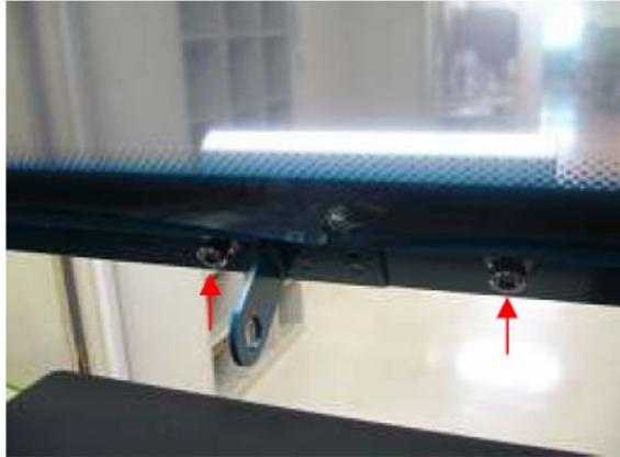
3. Remove the fixing jig for X-Axis Magtration Unit fixed by 3 screws inside the instrument.
