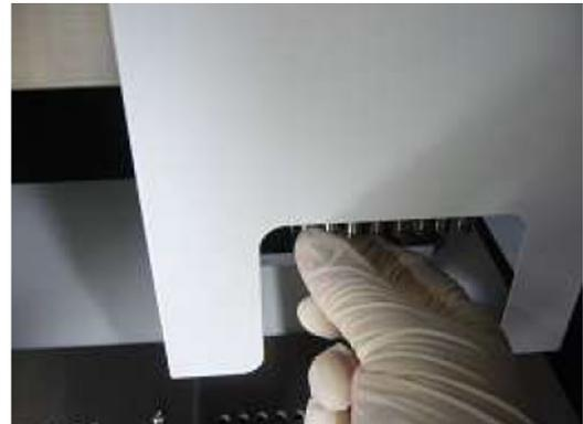
4. Use DN70 Tips to make the greased-O-rings fit.
