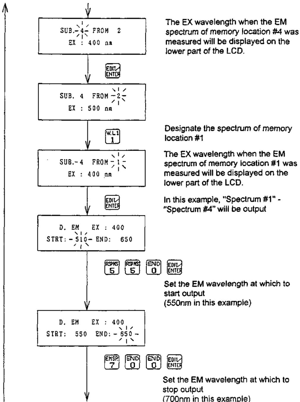
The EX wavelength when the EM spectrum of memory location #4 was measured will be displayed on the lower part of the LCD.
