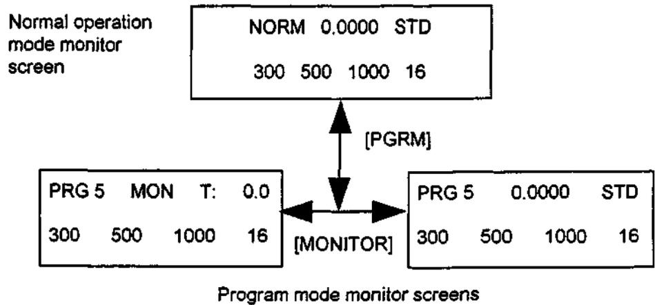
Figure 5-1 Switch between Normal Operation Mode and Program Mode
