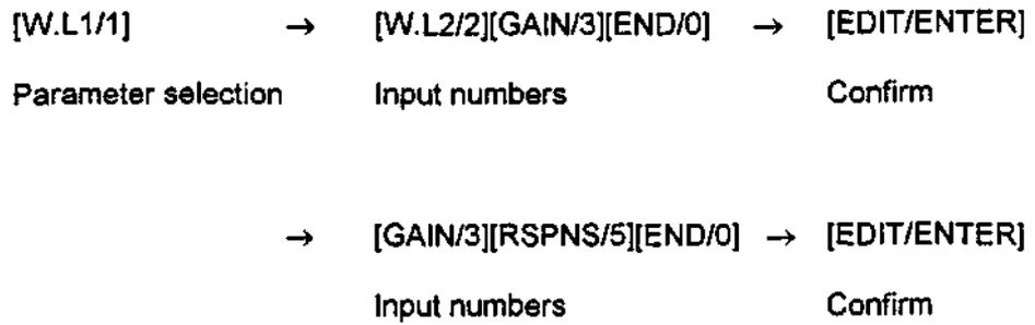
*Note 1: When [SHIFT][W.L1/1] is pressed, the screen will change to the preamp. output screen. When [MONITOR] is pressed, the screen will return to the screen shown in Fig. 3-1.*
