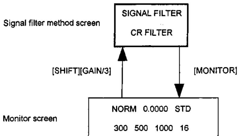
Figure 4-3. Signal Filter Method Display
