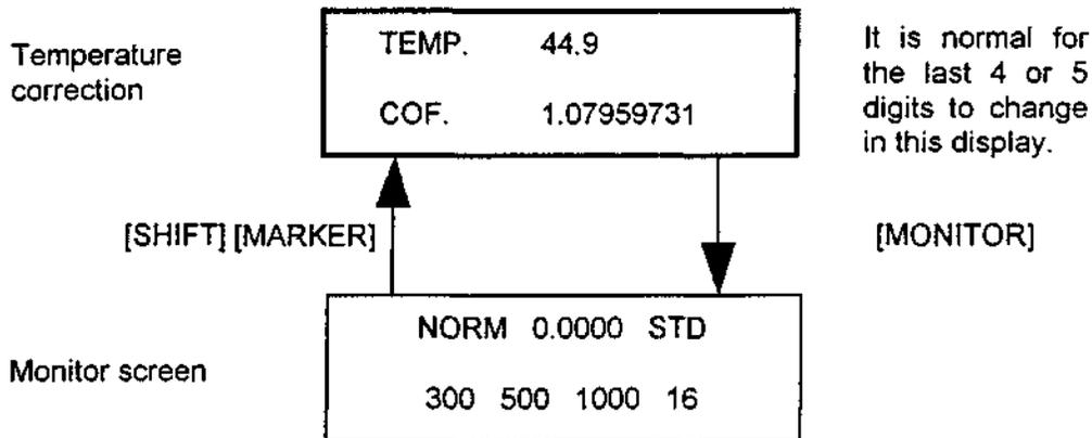
Figure 4-14 Displaying the Temperature
