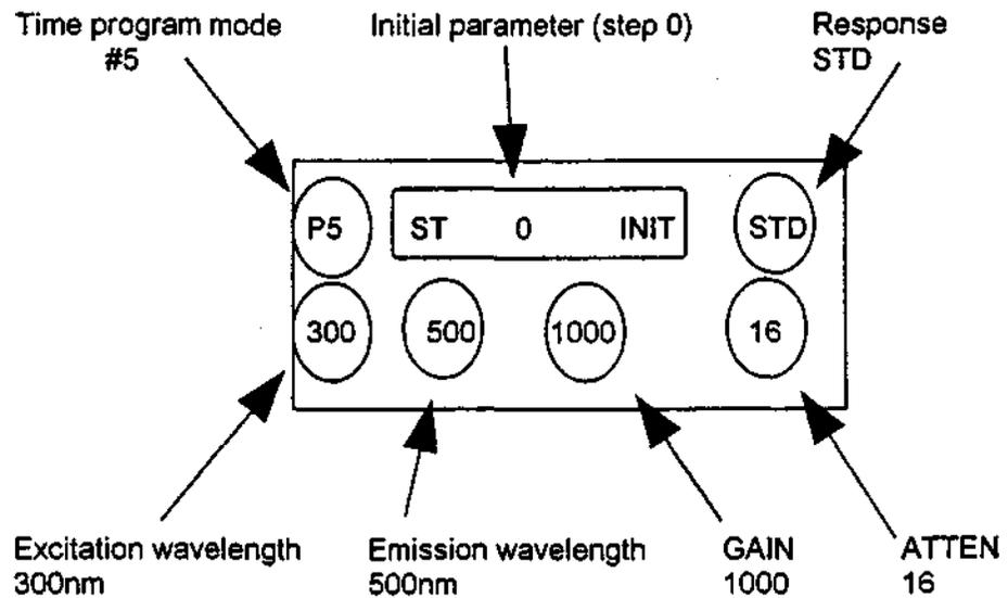
Figure 5-4 Explanation of the Initial Parameter Settings Screen
