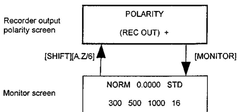
Figure 4-8 Setting of Recorder Output Polarity
