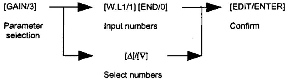
*Note: When [SHIFT][GAIN/3] is pressed, the screen will change to the signal filter setting screen.*
