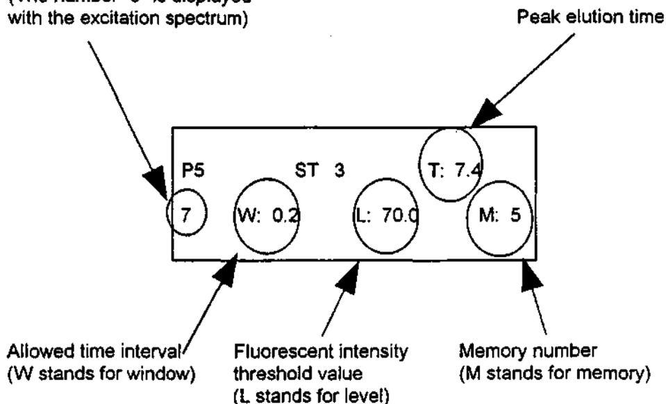
Figure 5-17 Example of Fluorescent Spectrum Measurement Settings
