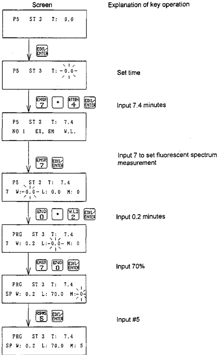
Figure 5-18 Input for Fluorescent Spectrum Measurement
