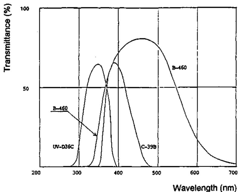
Figure 9-1 Characteristics of Excitation Filters
