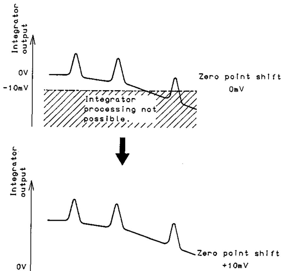
Figure 4-6 Method of Using Zero Point Shift
