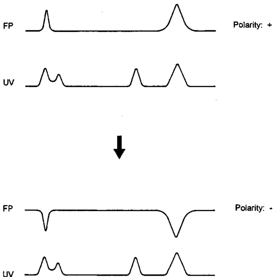
Figure 4-9 Method of Using Recorder Output Polarity
