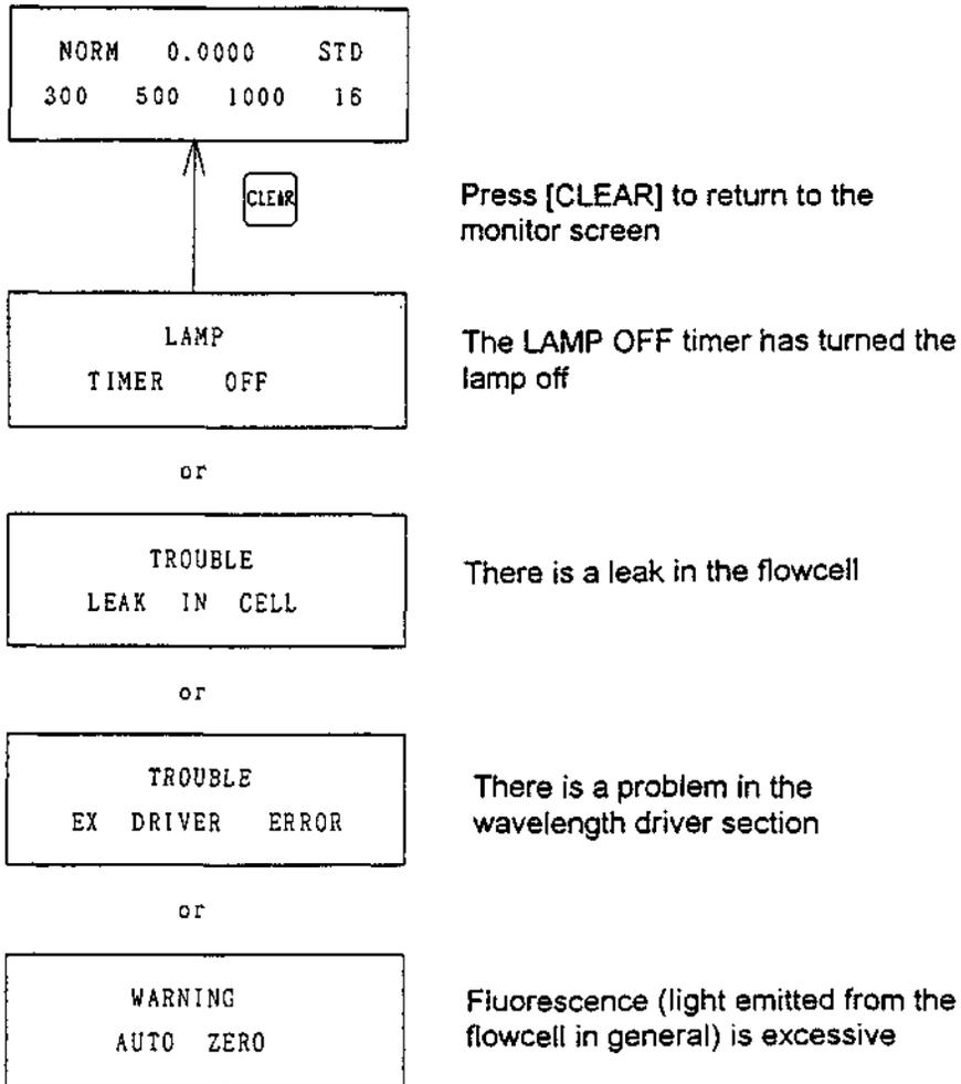
Figure 6-1 Possible Error Messages Displayed During Operation
