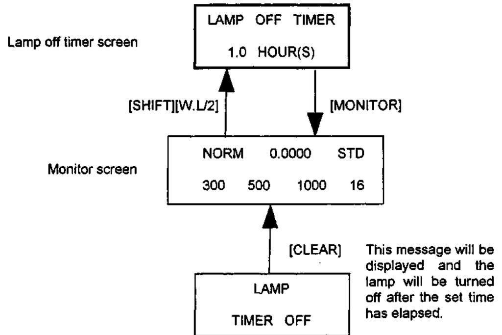
Figure 4-2 Operation of Lamp Off Timer
