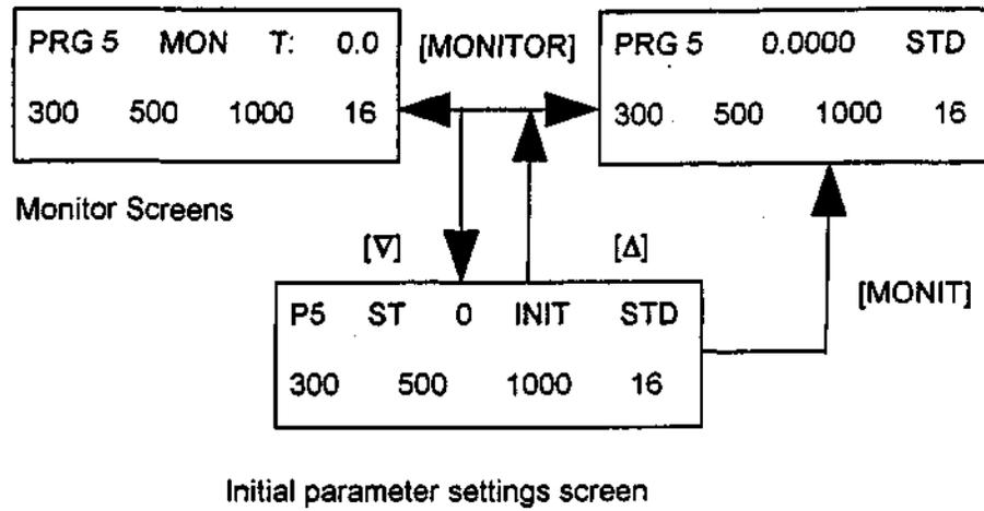
Figure 5-3 Initial Parameter Settings Screen
