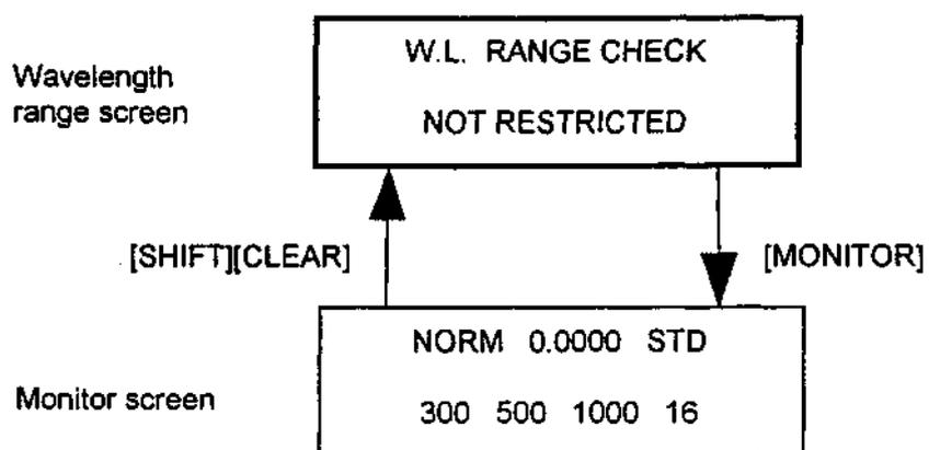
Figure 4-13 Setting the Wavelength Range
