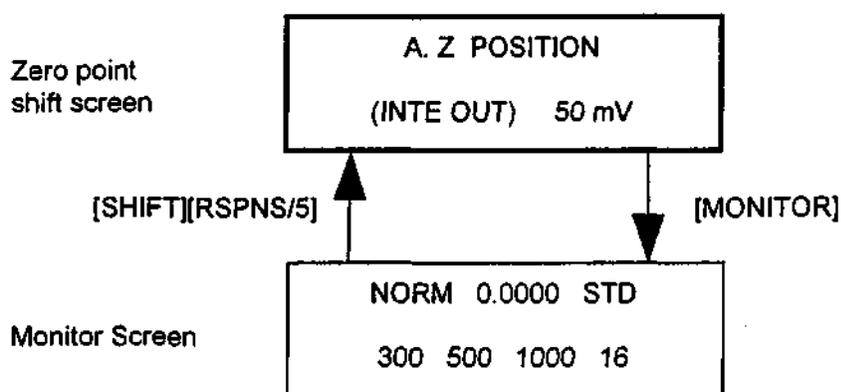
Figure 4-5 Setting the Zero Point Shift
