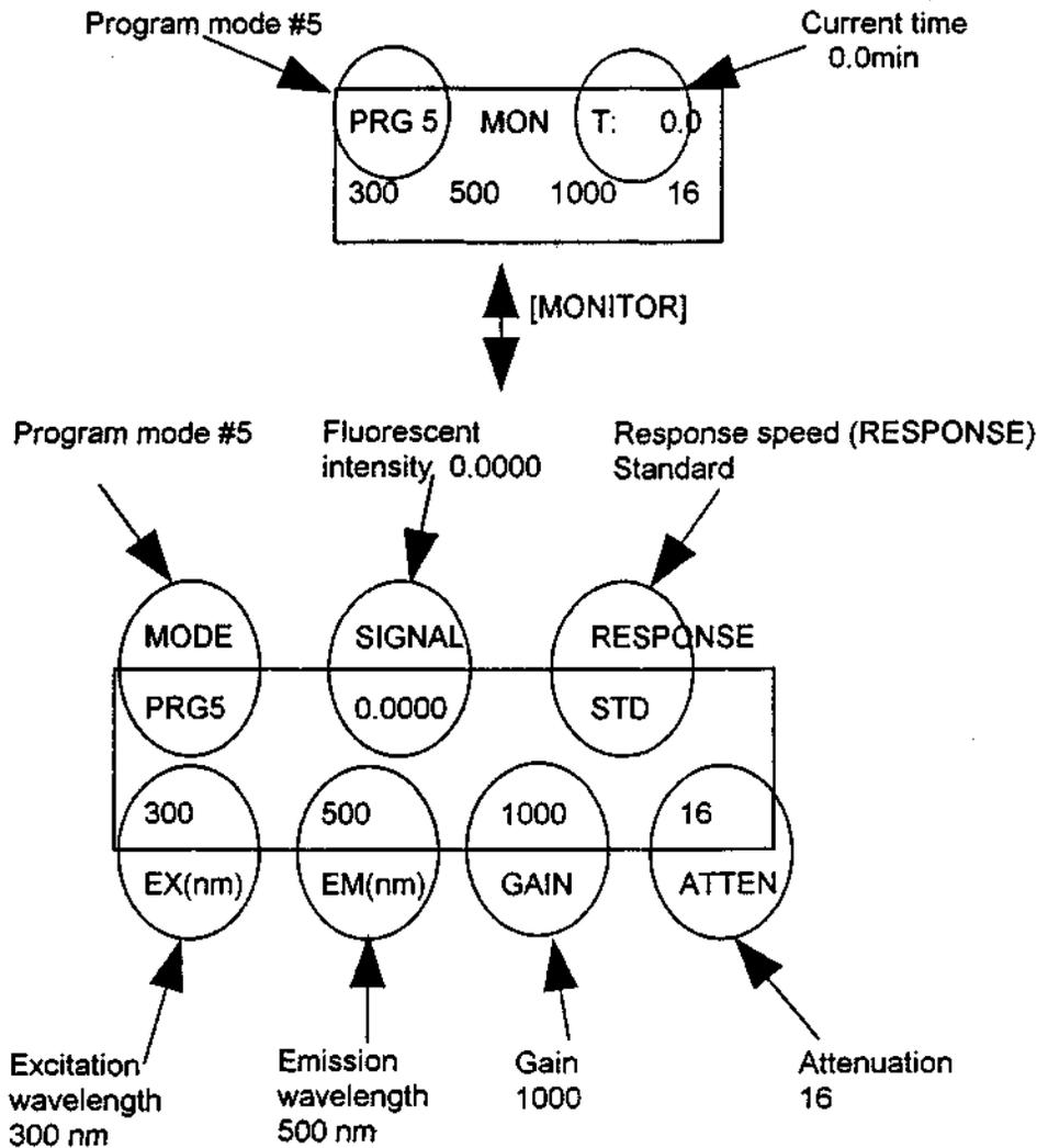
Figure 5-2 Explanation of the Program Monitor Screens
