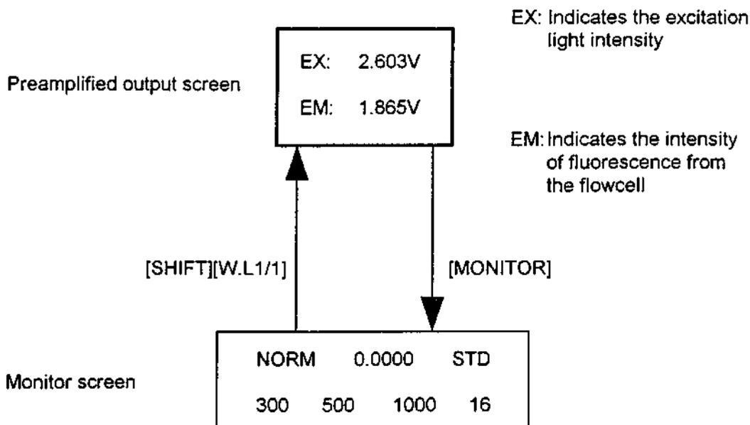
Figure 4-1 Displaying the Preamplified Output
