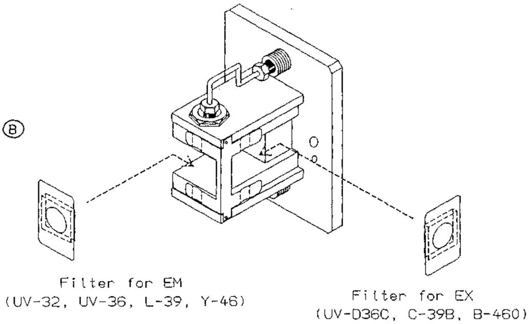
Figure 9-4 Flow cell cassette configuration
