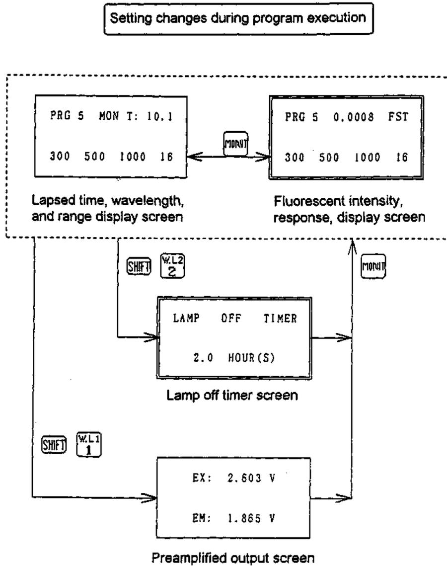
Figure 6-4 Changing Parameters During Program Execution
