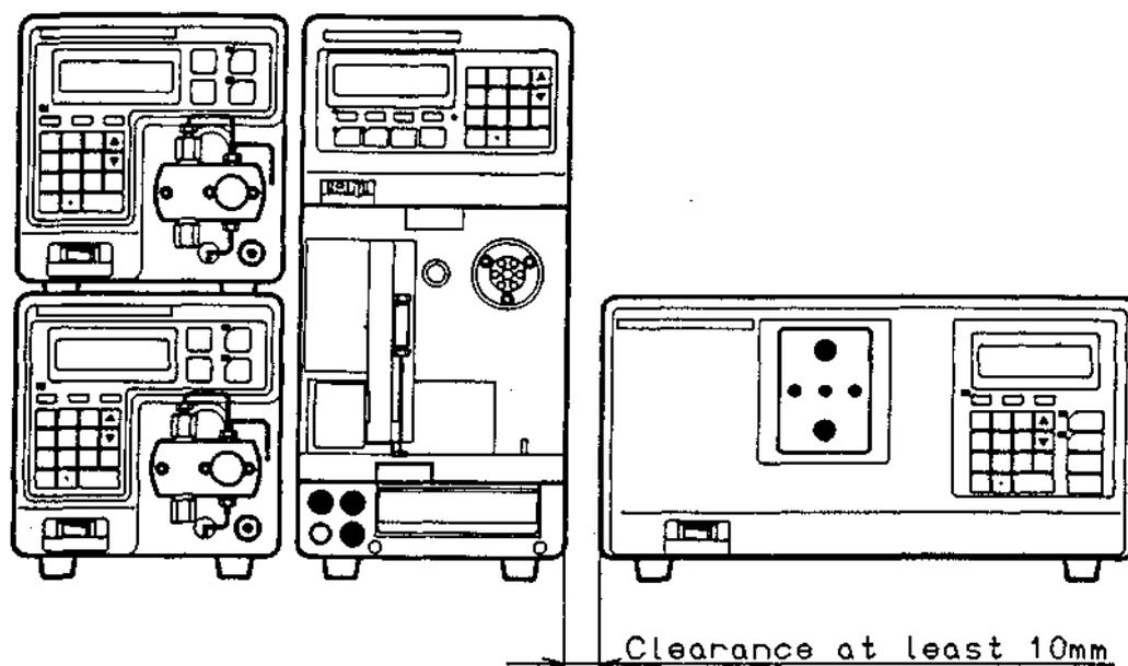
Figure 1-2 Arrangement Example
