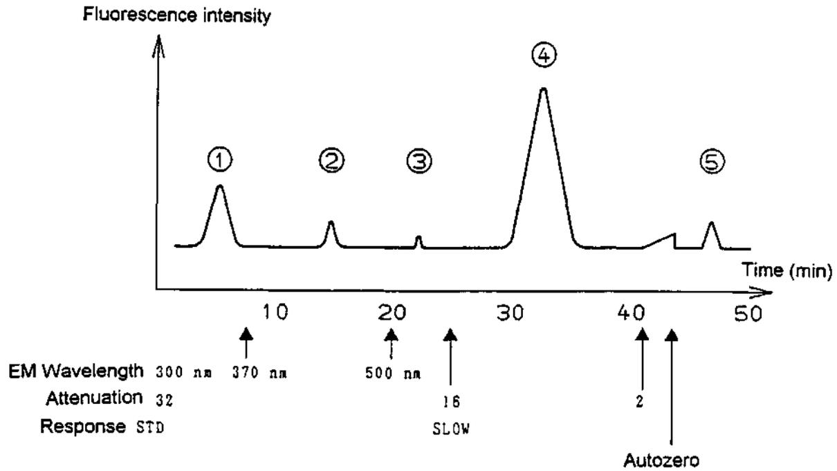
Figure 5-13 Chromatogram for Time Program Explanation
