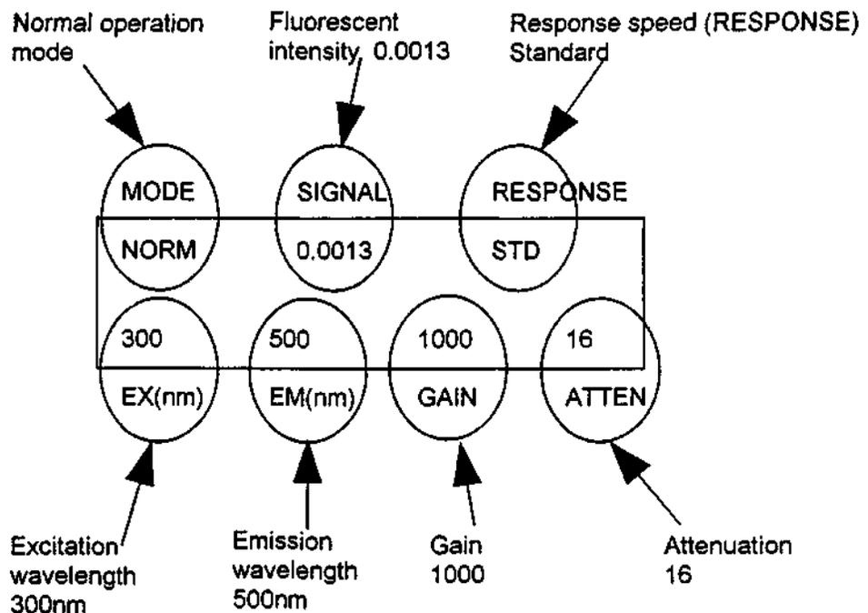
Figure 3-2 Description of the Normal Operation Mode Screen
