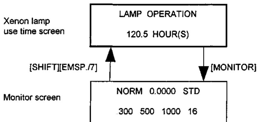
Figure 4-10 Displaying the Lamp Use Time
