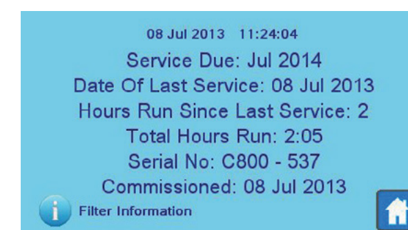
Full information screen with: next and last service date, hours run total and since last service, serial number, commissioning date, current time and date
