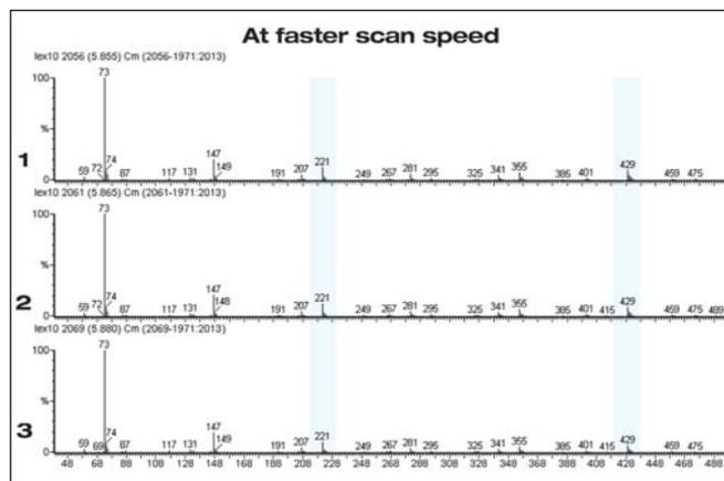
Figure 2. Better spectral fidelity with fast scan speeds, increasing confidence in results. Top and bottom figure with spectra acquired from (1) fronting, (2) apex and (3) tailing point along a chromatographic peak.
