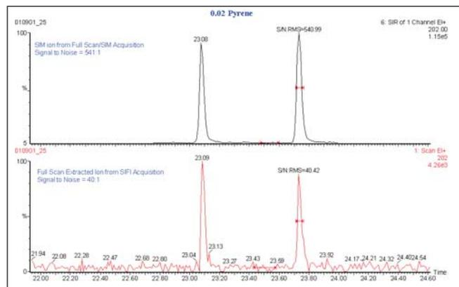
Figure 6. SIFI scanning ensures accurate identification, while simultaneously providing enhanced quantifiable sensitivity from the selected ion signal.
