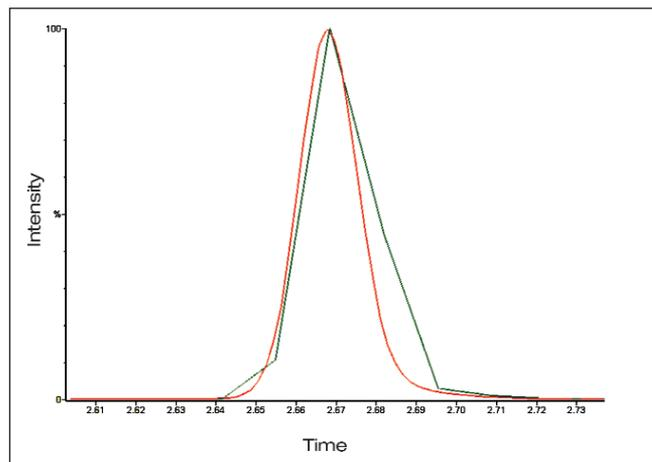
Figure 1. Chromatographic signal at fast scan speed (red) compared to slow scan speed (green).
