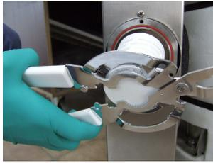
Fig. 45: Filter replacement: Removing the exhaust filter cartridge
