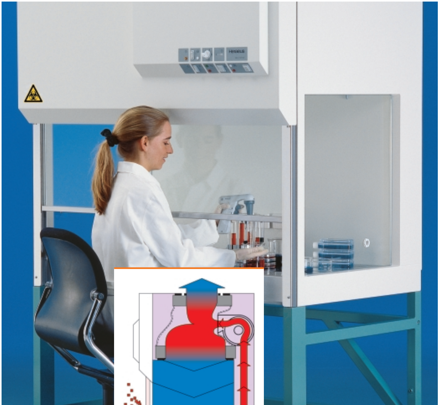
HERAsafe HS air-flow pattern
