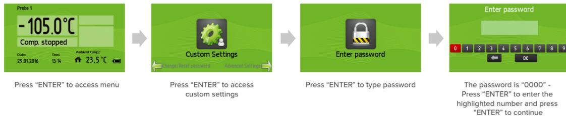
Press "Esc" to exit menu/go back. The display will return to the main screen after 1 minute of inactivity. When you have entered the custom menu successfully, you will have the following options:
