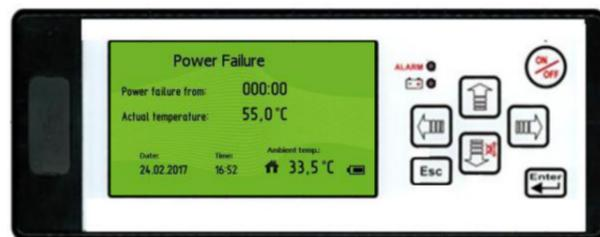
**Please note that during power failure, the cooling system will not be operational!** - When the power returns, the appliance will return to normal function. We highly recommend NOT to open the door during power failure, except for moving the products to another appliance or location. An open door will increase the temperature inside the chamber.
