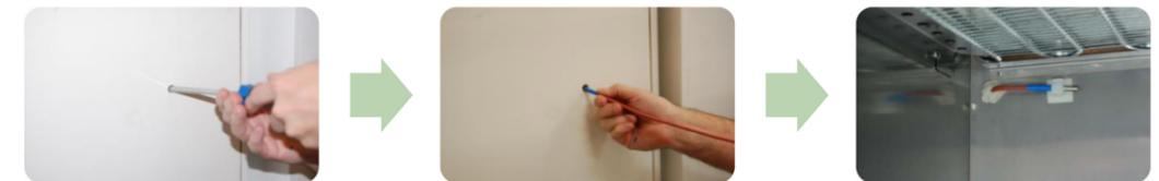
Never insert probes through the door, as this will danger the door gasket, increase the ice build-up and affect the temperature inside the appliance.
