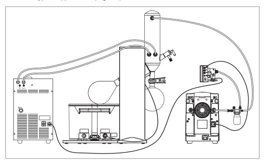
The connections to the Recirculating Chiller F-105, the Vacuum Pump V-100 and the Interface I-100 are described in the particular operating instructions in each case.
