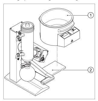
▶ Locate the heating bath (1) in the L-shaped cut-out in the Rotavapor base (2).
