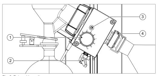
Fig. 2: Rotary drive unit
