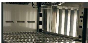
FIT S - light tubes installed in side walls
