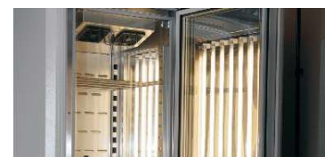
FIT DS - light tubes installed in door and side walls
