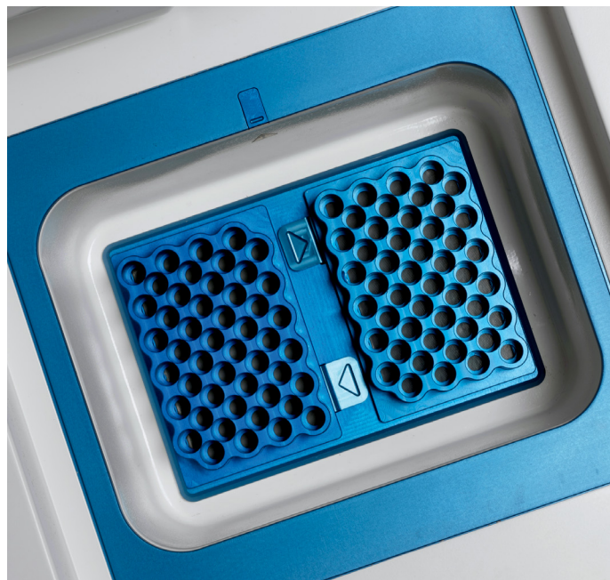
Fig 4. VIA Freeze™ Duo cryochamber loaded with two sample plates fitted on separate heat transfer pads with (A) two single 50 mL horizontal cryobag plates and (B) two single 48 × 2 mL cryovial plates.
