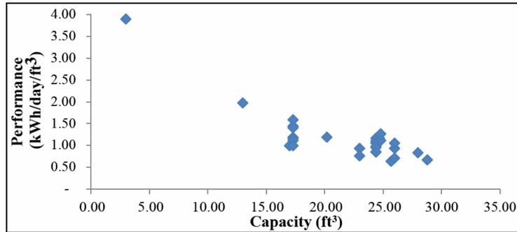
Note: The ULT freezers are operating at set point of –80°C and an ambient temperature of 25°C to 28°C.
