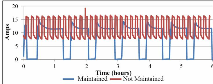
Table 4 depicts the conditions of two freezers that were evaluated to determine the effects of a thick dust on the filter and no dust on the condenser fins.
