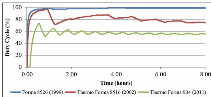
Figure 3 is a graphical representation of how age influences the energy consumption for maintained  $17.3\text{ ft}^3$  ULT freezers at a set point of  $-80^{\circ}\text{C}$  operating in ambient temperature ranging from  $23^{\circ}\text{C}$  to  $28^{\circ}\text{C}$ . As seen in the figure, for each year a freezer ages, there is an increase of approximately 3% in energy consumption, and an additional monthly release of  $8.75\text{ kg}$  of  $\text{CO}_2\text{e}$ .
