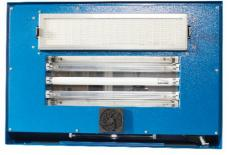
We recommend you change the HEPA filter after 1500 hours of operation. The Carbon filter should be repaced after 3000 h of operation (based on the default setting of 0.5 m/sec of the air flow. With less
