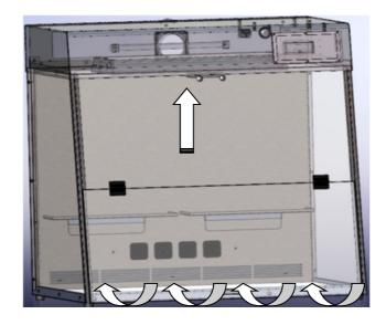
NOTE: Equipment in front of the air vents will block airflow.
