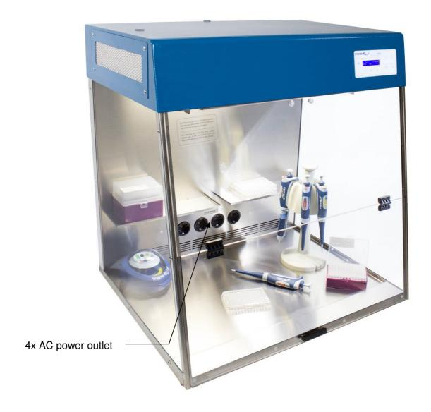
The 4 AC power outlets serve as power supplies for devices used inside the PCR chamber.
