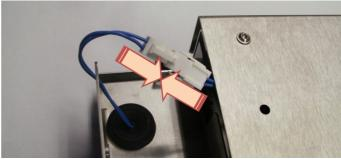
Slide the connection assembly into the cavity of the back panel.
