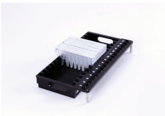
Figure 44. Placing the cartridges in the Deck Tray and pressing firmly to snap in place.
