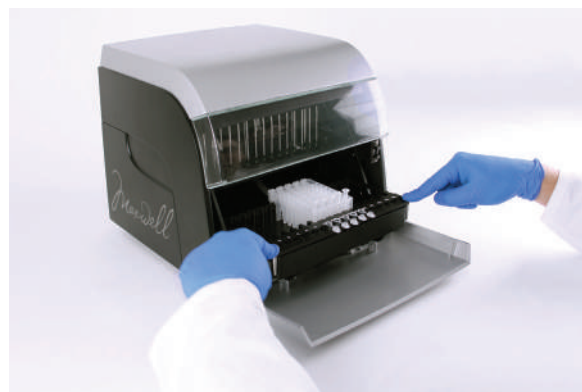
Figure 44. Placing the cartridges in the Deck Tray and pressing firmly to snap in place.
