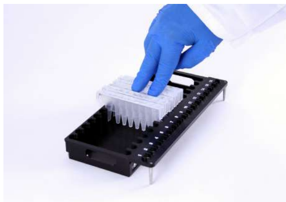
Figure 44. Placing the cartridges in the Deck Tray and pressing firmly to snap in place.
