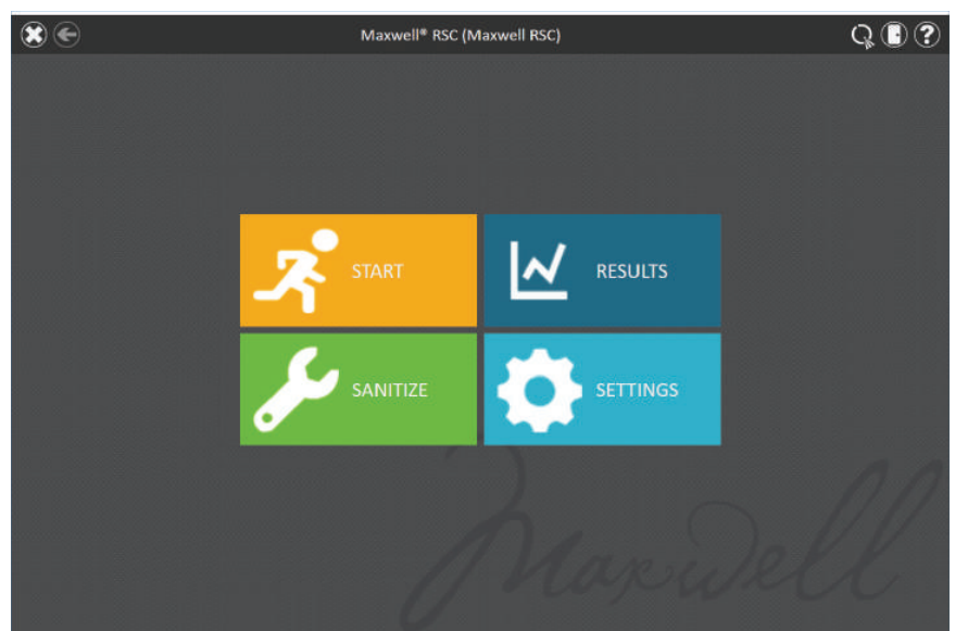
Figure 36. Maxwell® RSC 'Home' screen. Selecting the Start button begins the process of running an extraction method on the Maxwell® RSC Instrument.
