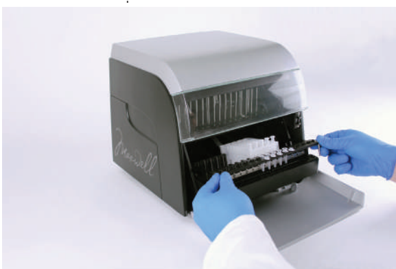
Figure 45. Placing the deck tray in the instrument.
