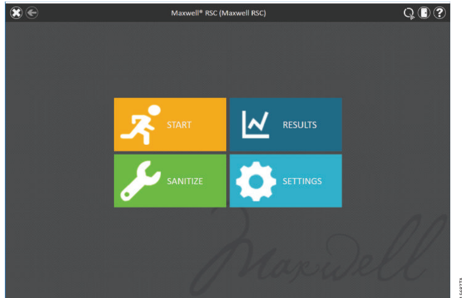
Figure 64. 'Home' screen. Selecting the Sanitize button begins the process for UV treatment of the Maxwell® RSC Instrument.
