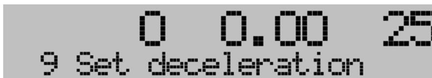
2. Select the desired curve by entering a digit between 1-9 on the numeric pad. Curve number 1 is the slowest and curve number 10 the fastest.
