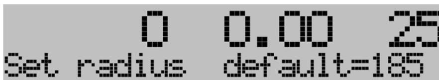
The default value is marked accordingly. You can either confirm the default value by pressing ENTER
