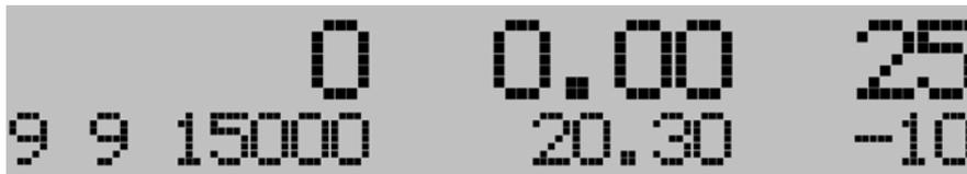
The top line shows the speed and the time. The temperature indicator displays the current temperature inside the rotor chamber. The bottom line shows the values for the last run.
