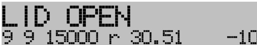
The top line shows the message “Lid open”. The bottom line shows the values for the last run.
