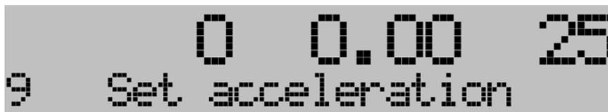
2. Select the desired profile by entering a digit between 1-9 on the numeric pad. Curve number 1 is the slowest and curve number 9 the fastest.
