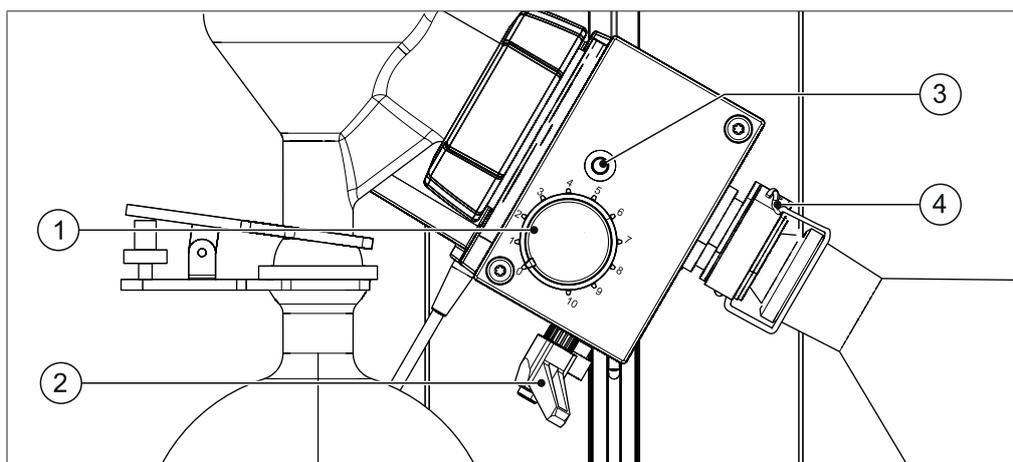
Fig. 2: Rotary drive unit
