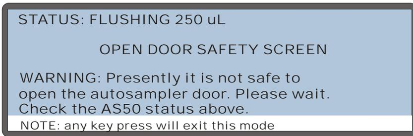
*Figure 3-8. Open Door Safety Screen: Not Safe to Open Door*
