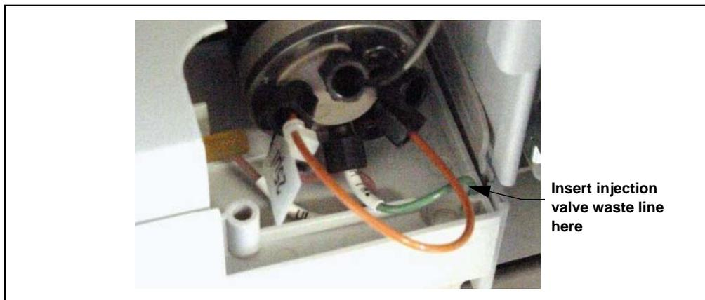
*Figure 5-12. Routing the Injection Valve Waste Line to the Drip Tray:
