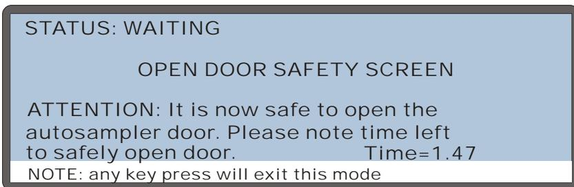
*Figure 3-9. Open Door Safety Screen: Safe to Open Door*
