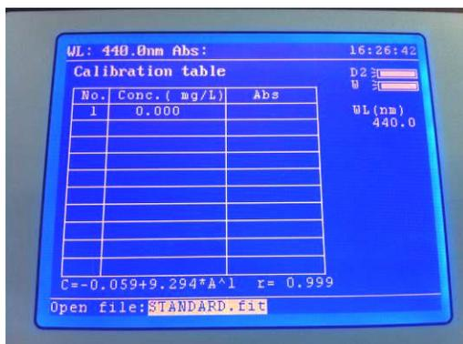
A standard curve can be opened from the instrument's internal memory to allow it to be re-used for sample quantification.
