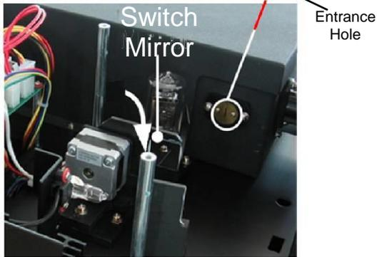
3. Whilst wearing cotton gloves remove the defective tungsten lamp and replace with a new one.
