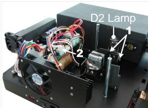
1. Unscrew the 4 screws on the spectrophotometer's top case (see 12.2.1) and remove the cover of the spectrophotometer.
