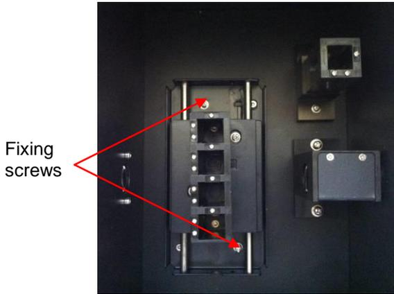
Unscrew the two fixing screws to undo the passive accessory. Lift out the passive accessory.
