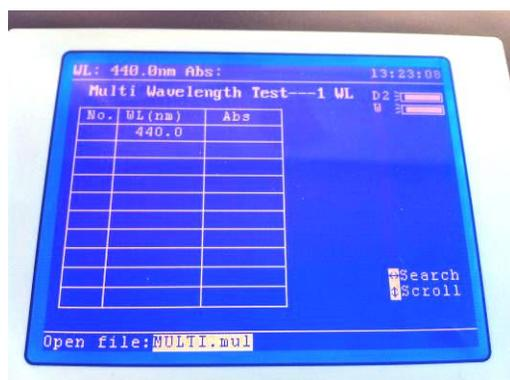
A method/result file can be opened from the instrument's internal memory.
