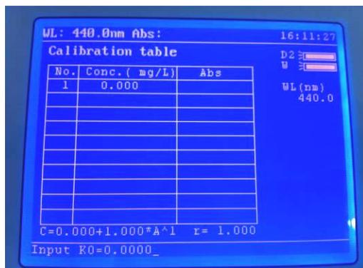
The user can manually enter the calibration curve constants by pressing the function key below the Params option. The user will be prompted to enter the constants that are required for the selected curve fit algorithm.
