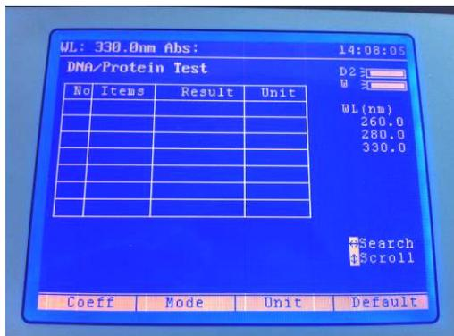
The DNA/Protein measurement mode enables measurement parameters to be changed. The four options at the bottom of the screen allow the user to edit the concentration calculation factors, select the measurement mode, select the units of the measurement and reset the modes settings to their default values. These options are selected with the corresponding function buttons.
