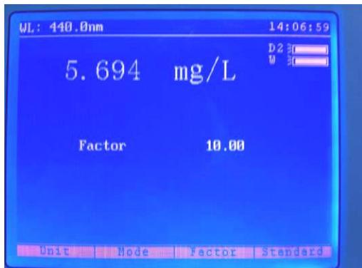
Remove the cuvette containing the blank solution and place a cuvette containing the sample to be measured in the sample chamber. Close the instrument lid and the concentration value will be shown on the screen.
