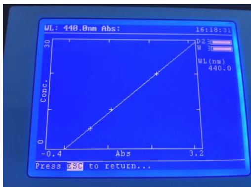
The standard curve can be viewed graphically by pressing the function key below the show curve option on the calibration table screen.
