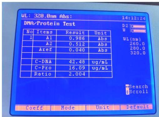
Ensure that a cuvette containing the blank solution is in the reference position in the sample chamber and insert the cuvette containing the sample solution into the sample position. Close the instrument lid and press the Start/Stop key on the keypad. Once the measurement is complete the determined results will be displayed in the DNA/Protein mode screen. Further samples can be measured in a similar manner.
