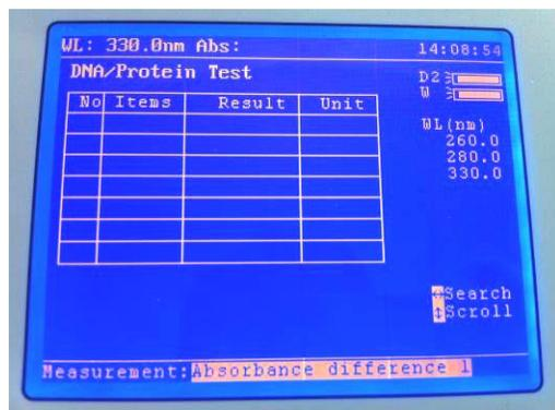
The DNA/Protein measurement mode includes two sets of calculations to calculate the concentration of nucleic acid and protein samples. The measurement mode option can be selected by pressing the function key below the Mode option. The options that are available are:-
