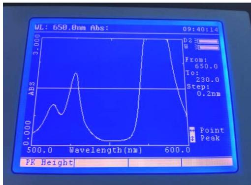
The photometric values of the measured spectrum can be viewed by pressing the function key below the Search option. The user can press the up and down arrow keys to move between the peaks in the scan that are above the threshold peak height. The user can alternatively press the left or right arrow keys to review each point in the scan in turn.
