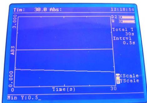
The instrument will display the full range scan after a measurement is complete. To change the displayed time range, press the left or right arrow keys. The start and end times can be entered using the numeric keypad. Press the Enter key to confirm. To change the displayed photometric range, press the up or down arrow keys. The minimum and maximum values can be entered using the numeric keypad. Press the Enter key to confirm.
