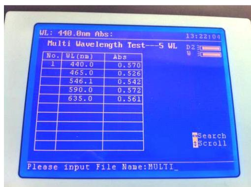
A method/result file can be saved to the instrument's internal memory.
