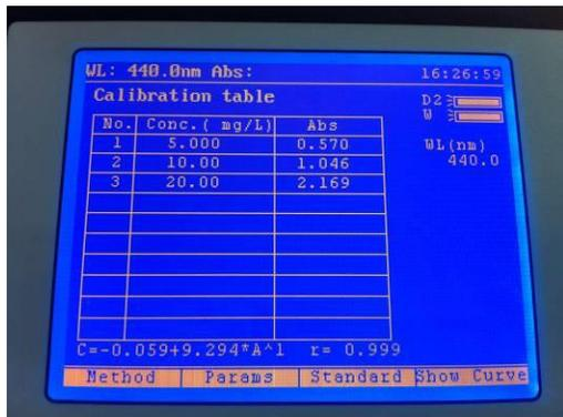
Once all standard solutions have been measured the new standard table and curve equation will be shown.
