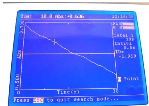
The photometric values of the measured kinetics scan can be viewed by pressing the function key below the Search option. The user can press the up and down arrow keys to review each point in the scan in turn.
