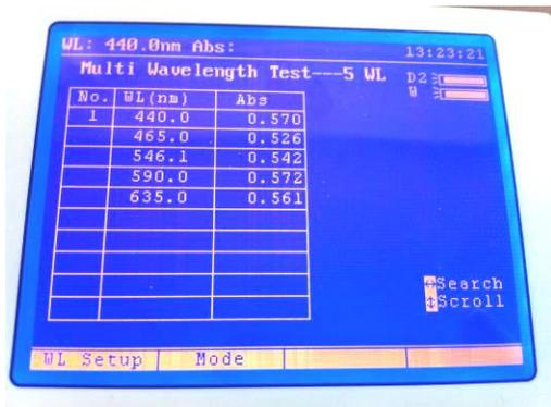
Insert a cuvette containing the sample to be analysed into the sample chamber and press the key below the sample measurement icon. The instrument will take a reading at each of the specified wavelengths the operating menu screen will then display the result of the selected measurement calculation and the photometric readings for each of the measured wavelengths.
