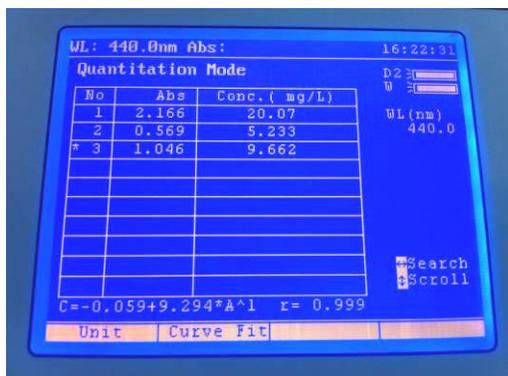
Ensure that a cuvette containing the blank solution is in the reference position in the sample chamber and insert the cuvette containing the sample solution into the sample position. Close the instrument lid and press the Start/Stop key on the keypad. Once the measurement is complete the determined result will be displayed in the quantitation mode screen. Further samples can be measured in a similar manner.
