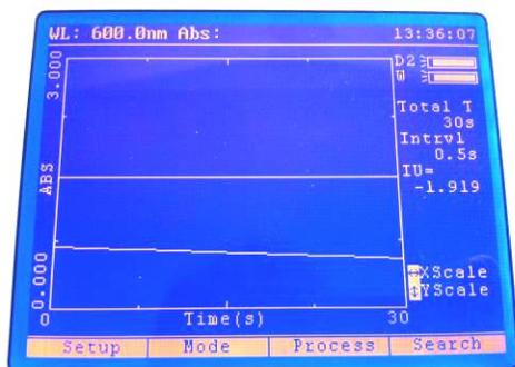
Insert a cuvette containing the blank solution into the reference position in the sample chamber and insert the cuvette containing the sample solution into the sample position. Close the instrument lid and press the Start/Stop key on the keypad. Once the measurement is complete the measured kinetics scan will be displayed on the screen.
