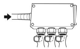
To disconnect the fluid lines, push on the button and pull the connector.
