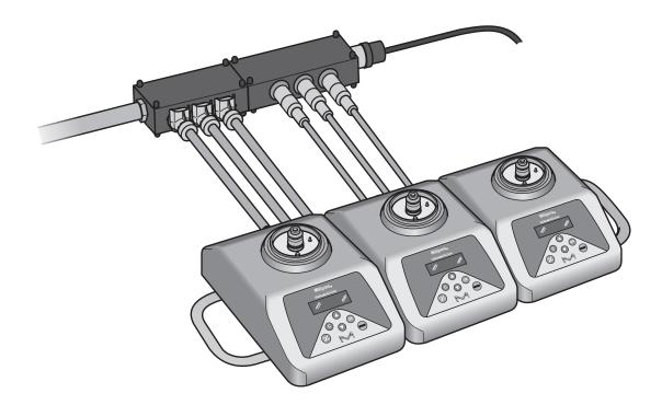
It is recommended to assemble the pumps together **before placing the system in the isolator**. The use of the tray facilitates the transfer of the assembled system to the isolator.
