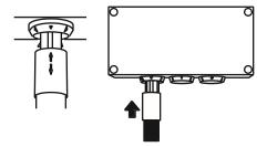
Connect the power supply to the electrical hub and tighten the connector.
