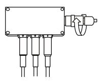
To disconnect the electrical cables from the hub, pull the cables out of the hub.
