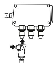
Insert the output tubing onto the stainless steel connector.
