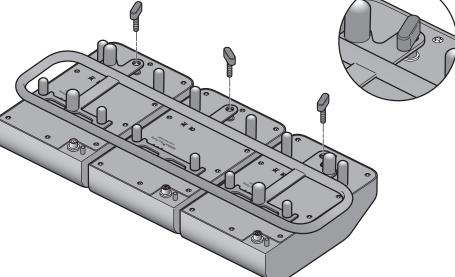
• Once the 3 pumps are assembled on the tray, connect the electric cables and fluidic tubes to each pump
