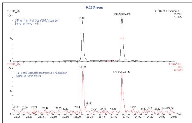
Figure 4. SIFI scanning ensures accurate identification, while simultaneously providing enhanced quantifiable sensitivity from the selected ion signal.
