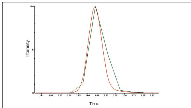
Figure 3. Chromatographic signal at fast scan speed (red) compared to slow scan speed (green).
