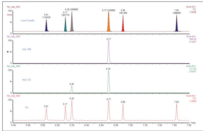
Figure 5. TIC (total ion chromatogram), extracted ions (121 and 106), and TIC integration.
