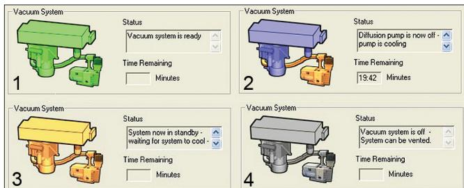
Figure 2. Diffusion-pump venting sequence.
