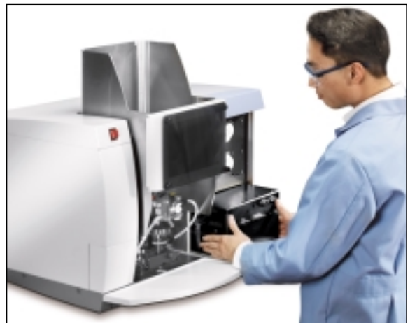
Figure 2. User-replaceable electronic module simply slides out for easy replacement.
