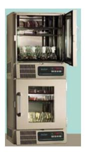
Two Innova 4200/4230 shakers can be stacked using the optional stacking kit.
