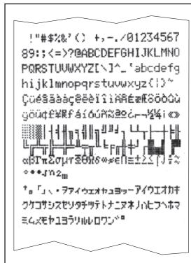
The RS-P42 is equipped with a self-test which automatically prints out the character set of the printer.
