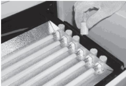
9. Insert the new starter into the holder and rotate clockwise.
