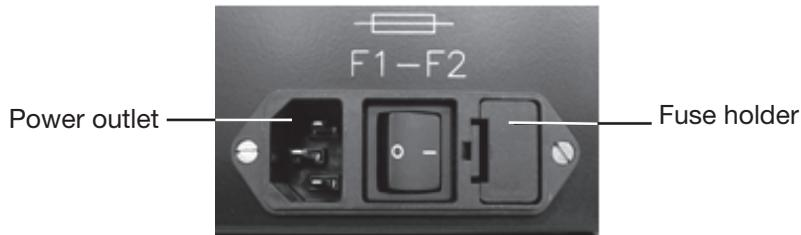
This unit is protected by two fuses (5 x 20 mm, 2A Slo-Blo). The fuses are located in the left side rear of the universal hood, in a fuse holder housed in the power entry module.
