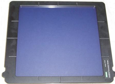
The XcitaBlue conversion screen is held in place by adhesive-backed edge guides. After the edge guides are installed, the conversion screen remains centered and will not slide, even if you close the drawer rapidly.
