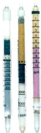
Figure 28: Example of chemical indicator tubes
