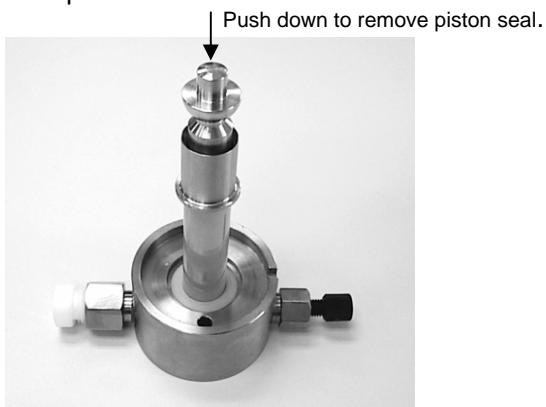
Figure 32 Ceramic Piston into Cavity
