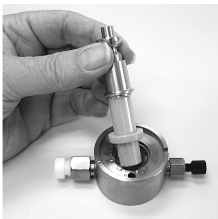
Figure 33 Piston Seal Removal
