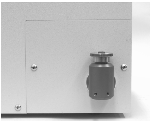
Figure 5 Internal Mixer in Place
