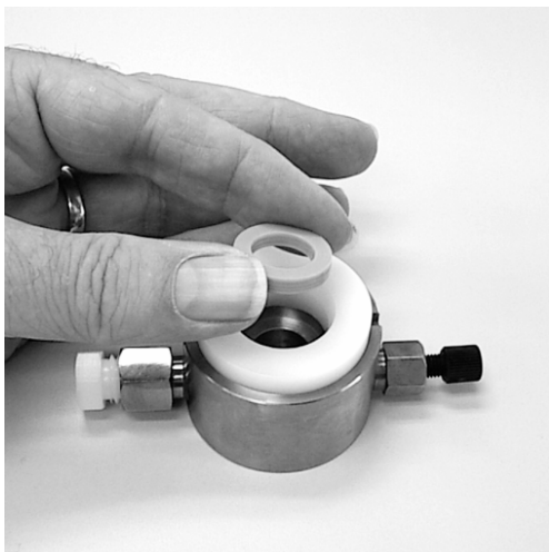
Figure 38 Inserting piston seal in tool
