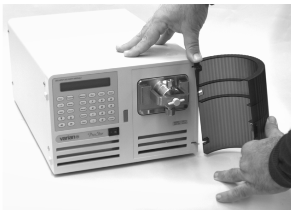
Figure 21 Installing the Door on the ProStar 210 Pump
