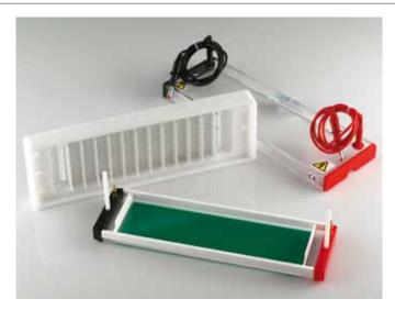
Gel units, horizontal, Thermo Scientific ABgene Electro-Fast® Stretch
