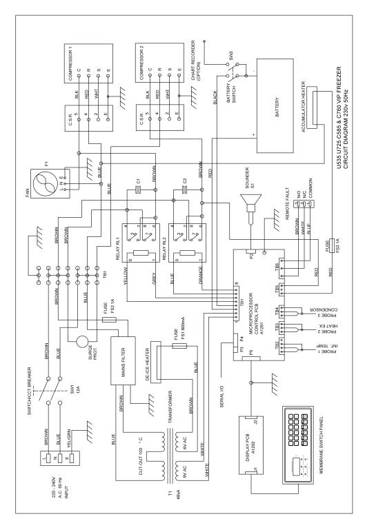
Figure 10: Circuit Diagram/Schematic for U535, U725, C585 & C760 Models (230V, 50Hz)
