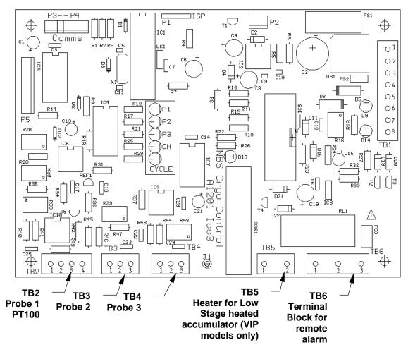
Figure 7: Main Control Board Components & Terminal Layout
