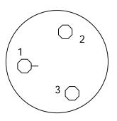
The freezers are provided with an alarm monitoring socket at the rear of the freezer and a matching plug for external monitoring purposes. This plug can be connected either to a central monitoring system or to a remote alarm via an auto-dialer. The configuration of the socket is shown in Figures 5 & 6 as viewed from the rear of the freezer.
