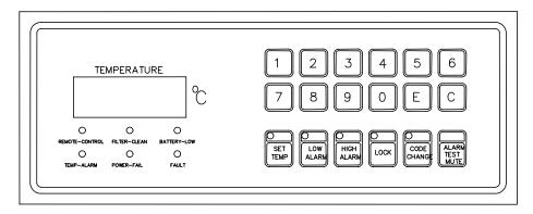
Figure 4: Display Panel & Keypad
