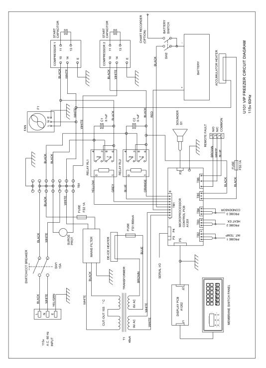
Figure 11: Circuit Diagram/Schematic for U101 Model (115V/220V, 60Hz)
