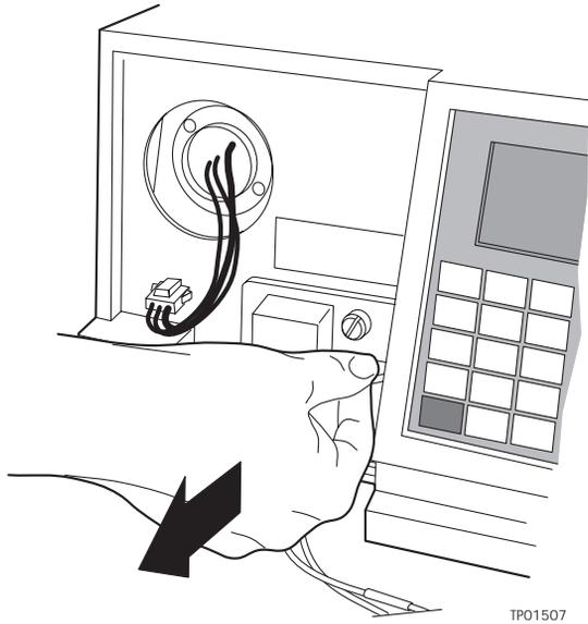
Figure 4-3 Removing the Flow Cell Assembly
