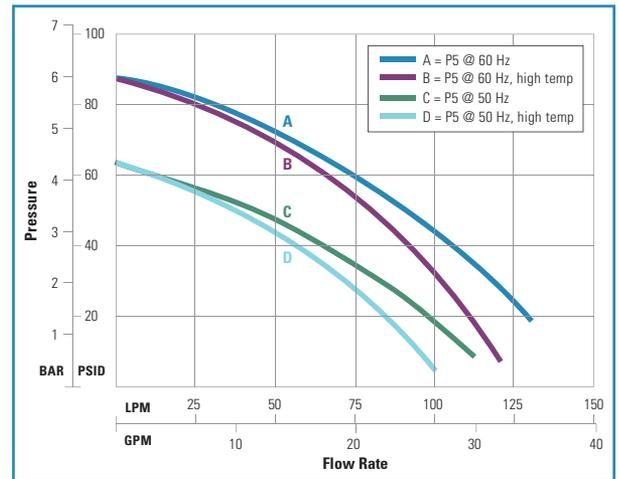
\*Pressure values for turbine and centrifugal pumps are differential pressures between the inlet and the outlet of the unit. Cooling capacity based on units with P2 pumps with no backpressure. Other pumps will affect cooling capacity performance.
