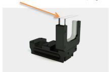
This holder is designed for use with a 50mm X 10mm optical glass cuvette.
