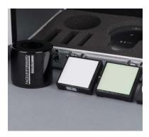
The black trap and white tile are used each time the instrument is calibrated. The green tile is used to perform an optional diagnostic test.
