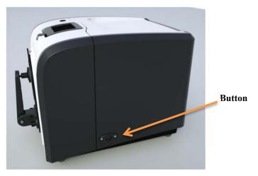
Depress these buttons, and slide the case toward the back of the instrument, to open the transmission compartment. Reverse the process to close the transmission compartment. The case will lock in the Open and Closed positions:
