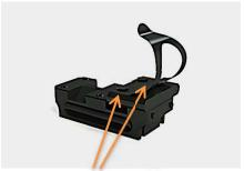
Two thumb **screws** provide the ability to adapt the holder to samples of varying thicknesses.
