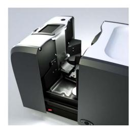
"Total" transmittance measurements are made with the white Spectralon® plaque in place at the front aperture plate and the sample placed against the sphere opening.
