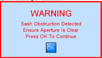
Remove the obstruction and press "OK". This will reset the system and the sash will close.
