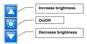
By pressing the "Up" or "Down" arrows you can adjust the brightness. Pressing the "Lighting" icon will turn the light off. Pressing the icon again will turn the light on.
