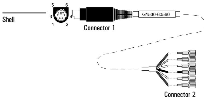
**Figure 24. Analog cable, general use (part no. G1530-60560)**
