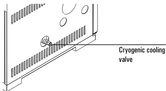
**Figure 18. Location of cryogenic cooling valve**
