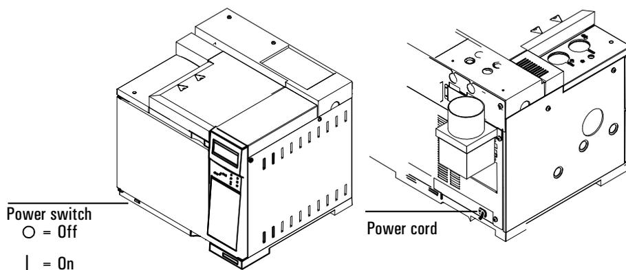
**Figure 9. Power switch and power cord locations**
