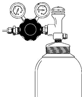
**Figure 3. Two-stage pressure regulator**
