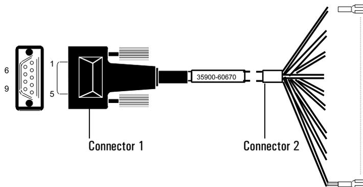
**Figure 25. Remote start/stop cable pin-outs, general use (part no. 35900-60670)**
