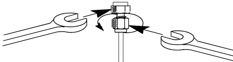
Tightening SWAGELOK nuts by this procedure provides a leak-proof, torque-free seal at all tubing connections.
