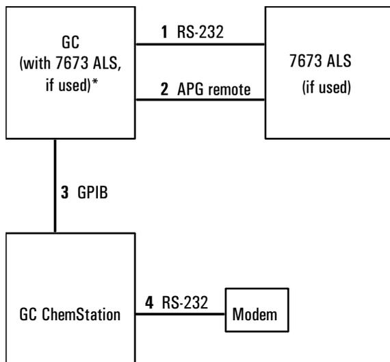
\* The 7683 controller is internal to the 6890 Plus GC. The G2613A Injector and the 2614 tray plug directly into the GC.
