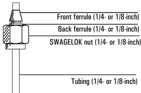
2. Make sure that the front ferrule is touching the inlet, and then slide the SWAGELOK nut over the ferrule and tighten it finger-tight.
