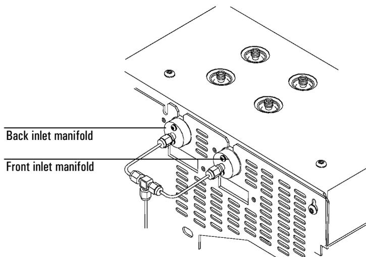
The GC in this figure has the front and back inlets plumbed with the same carrier gas.
