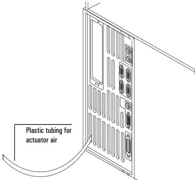
**Figure 19. Location of valve actuator air tubing**
