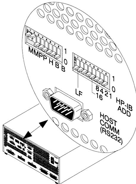
Figure 28. 7673 ALS switch location and correct configuration
