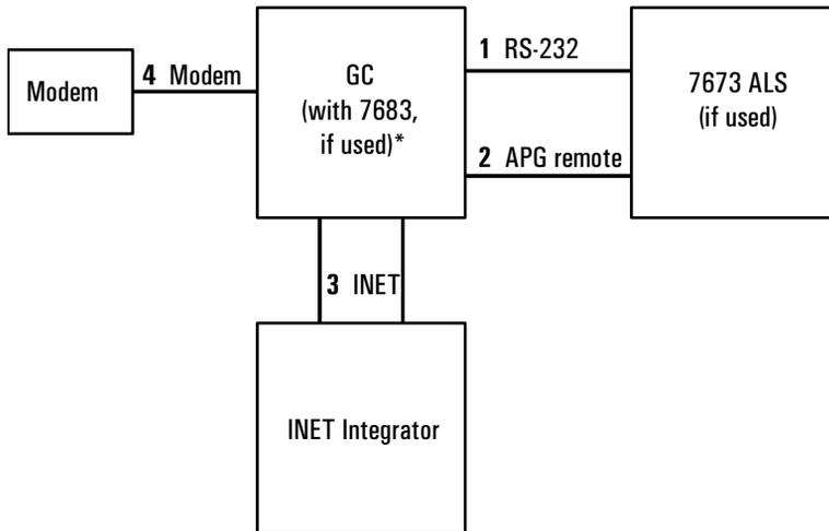
\* The 7683 controller is internal to the 6890 Plus GC. The G2613A Injector and the 2614 tray plug directly into the GC.
