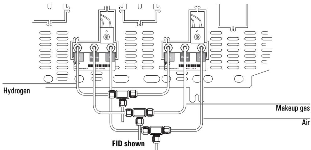
**Figure 14. Connecting tubing to an EPC detector**
