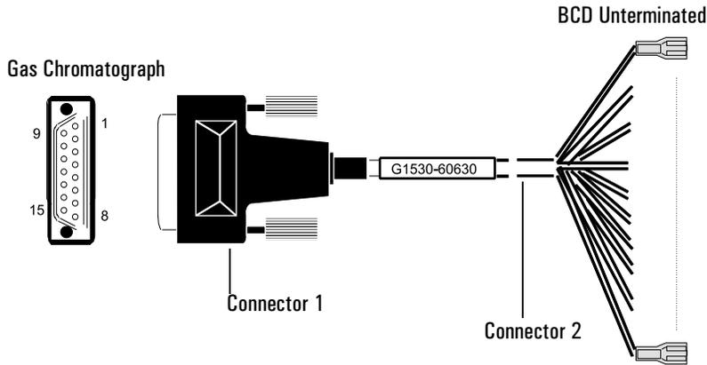
**Figure 26. BCD input cable, part no. G1530-60630**
