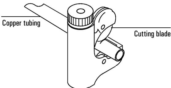
**Figure 10. Tubing cutter**
