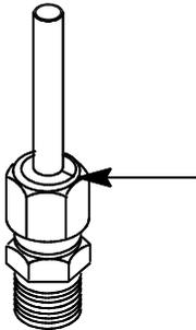
5. If you are using 1/8-inch SWAGELOK fittings, while holding the fitting steady with the other 7/16-inch wrench, tighten the fitting 3/4 of a turn. If you are using 1/4-inch fittings, tighten them 1 1/4 turn.
