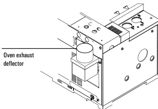
**Figure 8. Correct position of the oven exhaust deflector**
