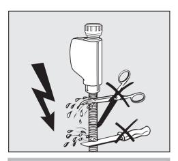
The inlet hose must **not** be shortened or damaged in any way (see illustration).
