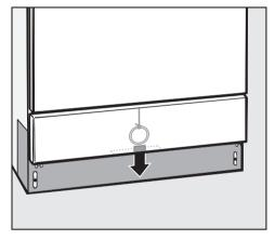
■ The emergency release cord is located at the bottom of the machine behind the service panel. Pull it downwards to open the door.
