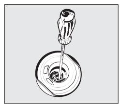
The dosage adjuster in the opening has settings adjustable from 1 to 6 (1-6 ml). It is set to 3 (3 ml) at the factory.
