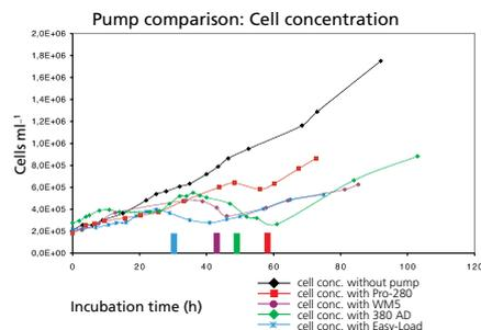
With the pump-head Pro-280 cell death was observed only after 56 hours whilst with the Easy-Load<sup>®</sup> pump-head death occurred already after 29 hours.
