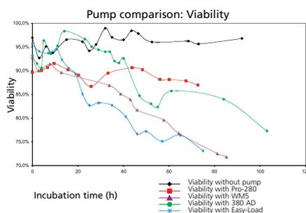
With the pump-head Pro-280 a viability of 87% was observed after **56 hours**. With the Easy-Load head a viability of only 72% was observed already after 29 hours.
