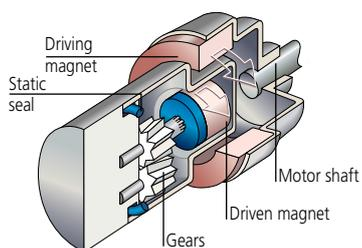
The two magnets couple automatically such that the driving magnet turns the driven magnet and gears without physical contact.
