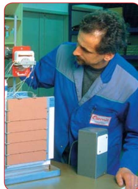
Long-term determination of environmental influences on asbestos-cement
