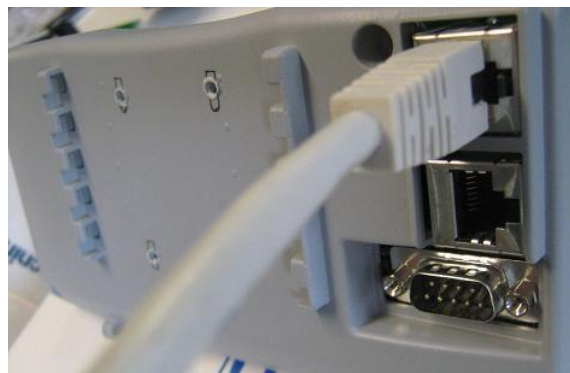
FIGURE 4.2.8.1. Ethernet cable connection to CPU
