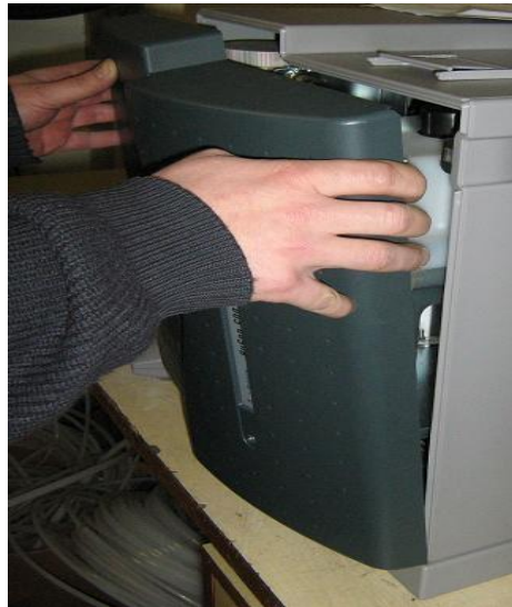
FIGURE 4.2.3.1. Removal of the front panel
