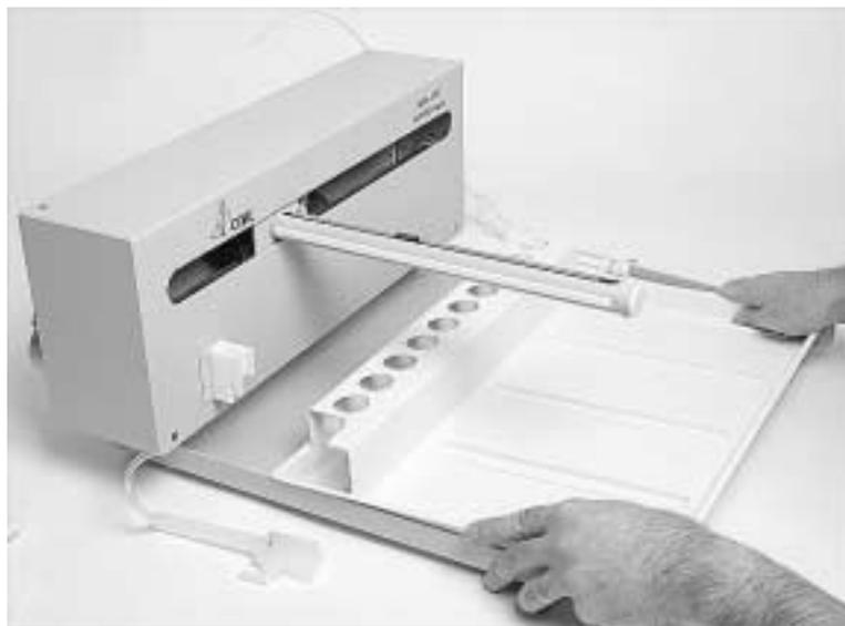
**Figure 3-11.** Removing the tray.
