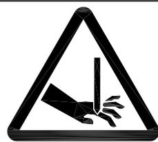
Pinch point on X, Y, Z axis movement.
