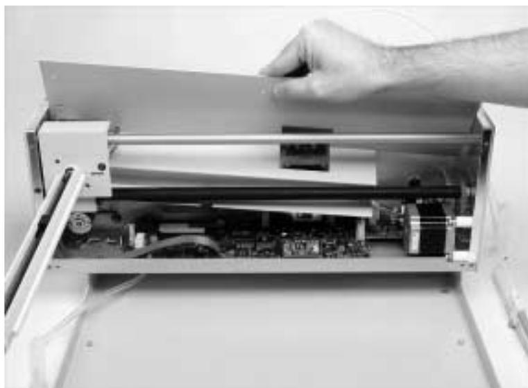
**Figure 3-15.** Removal of inner shield.
