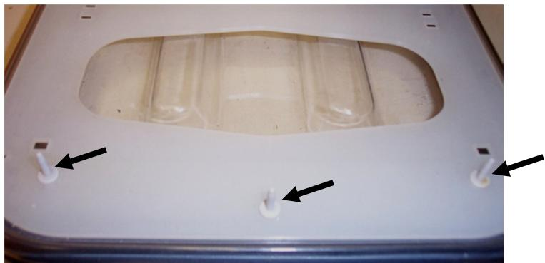
**Figure 12.** Locating pins correctly installed for additional standards rack.
