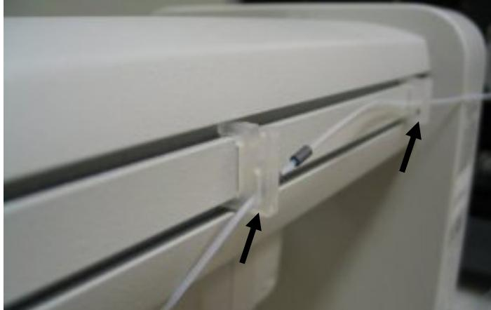
**Figure 16.** Location of tube-retaining clips.
