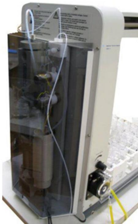
**Figure 21.** Agilent SPS 3 autosampler with optional Diluter installed.
