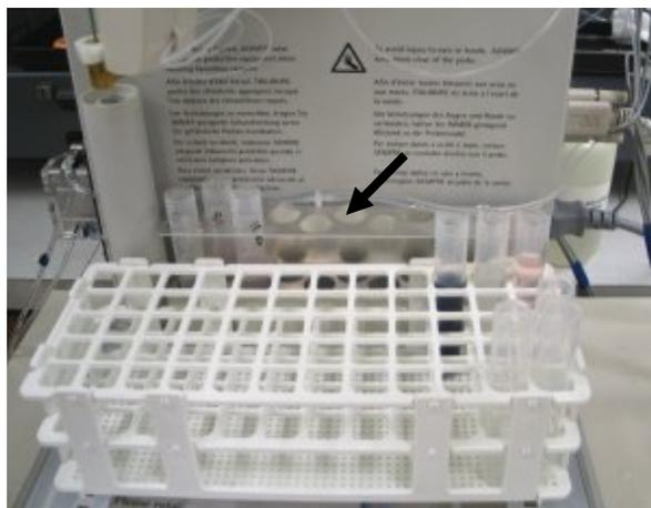
Figure 13. Standards rack installed on Agilent SPS 3.
