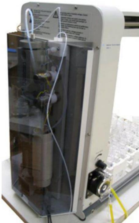
**Figure 21.** Agilent SPS 3 autosampler with optional Diluter installed.
