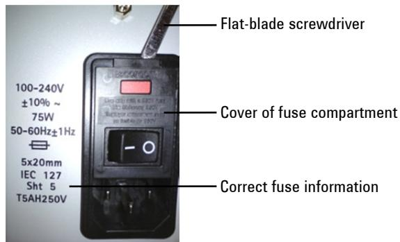
**Figure 18.** Opening the flap of the fuse compartment.
