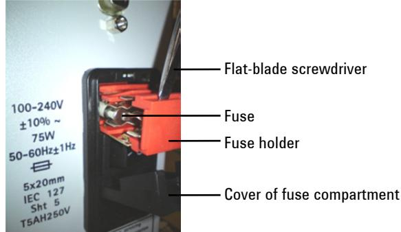
**Figure 19.** Sliding the fuse holder out of the compartment.
