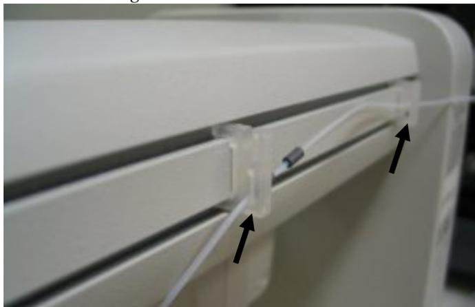
**Figure 16.** Location of tube-retaining clips.
