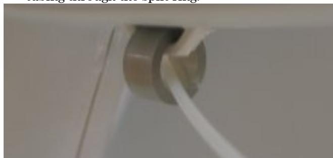
**Figure 15.** Routing the tubing through the split ring.
