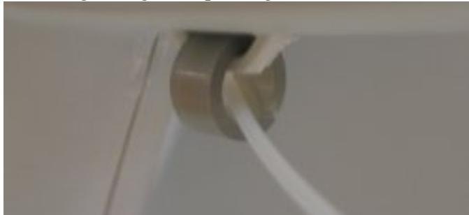
**Figure 15.** Routing the tubing through the split ring.
