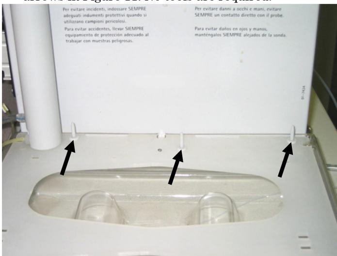
**Figure 11.** Standards rack locating pins correctly installed.
