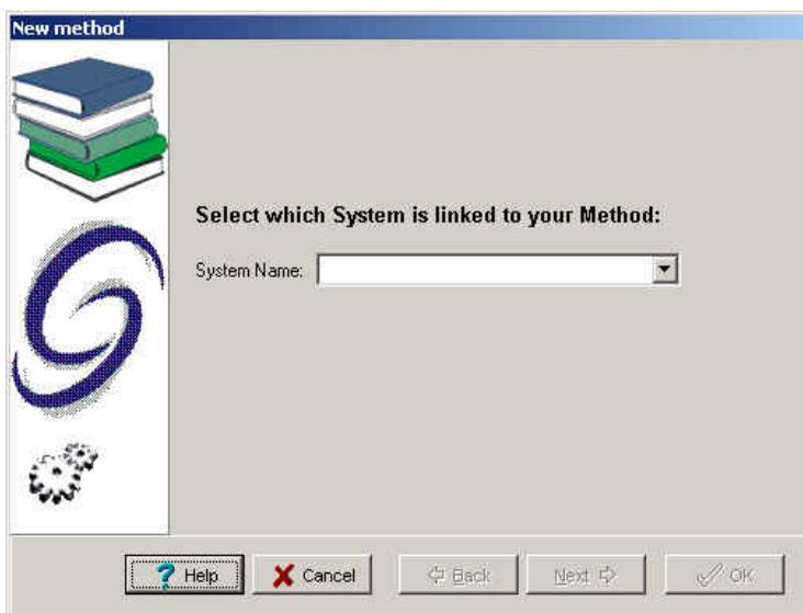
2. Choose the system (chromatograph) associated with the method. A method is created for a particular system. When starting an acquisition, the name of the system that performs the acquisition must be correct, since method access is limited only to those methods associated with this system.
