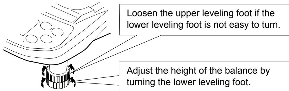
After adjusting the height of the balance, tighten the upper leveling feet if a rattling of the leveling feet occurs.
